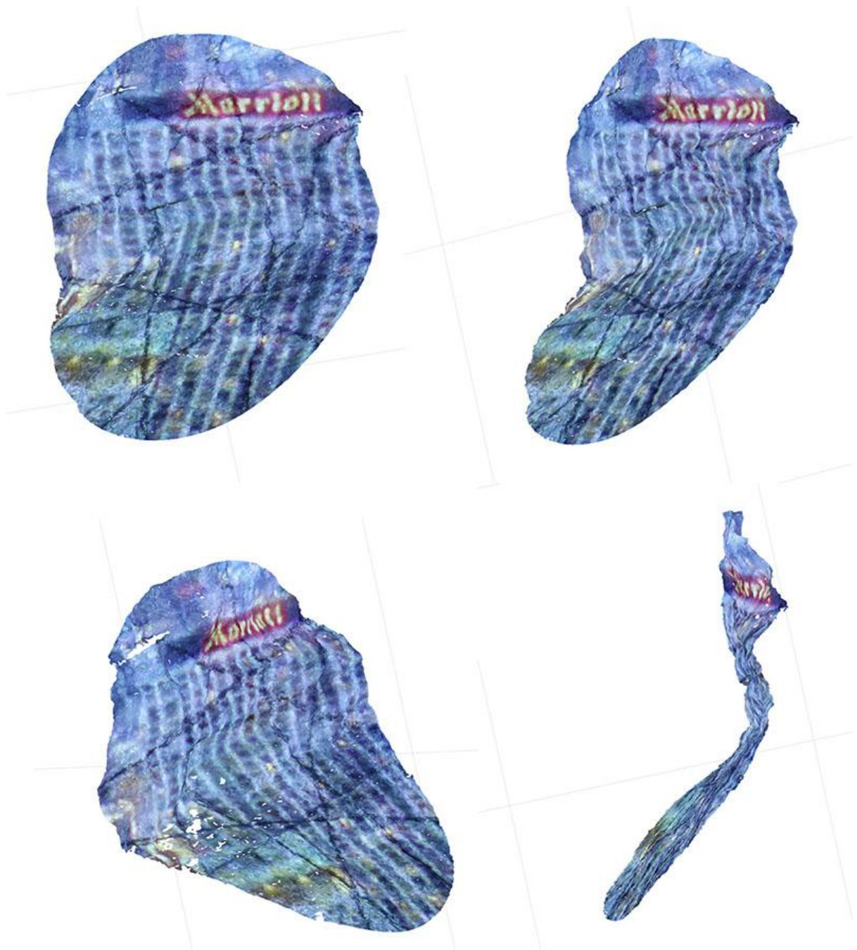
Figure 6. Images from different angles of the reconstructed core surface from the three-dimensional point cloud
