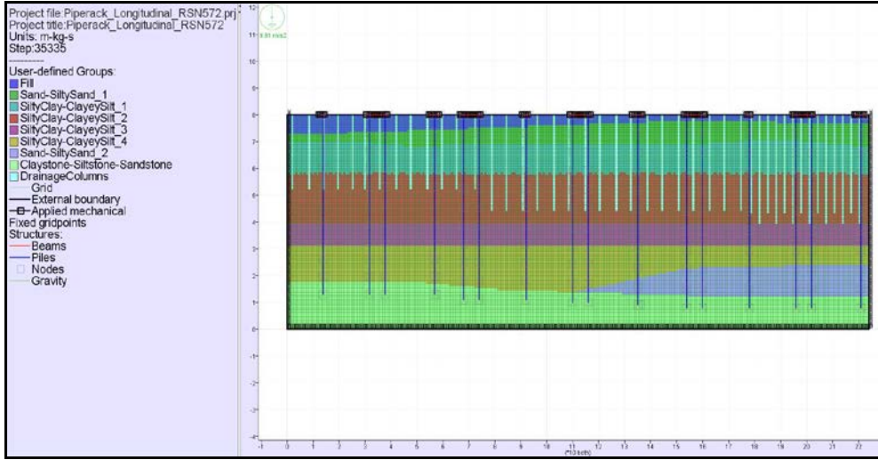
Fig. 1 - The drain columns and barrette foundations in the soil model for longitudinal cross-section
