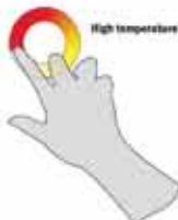
Single controls include just one button and a surrounding touch pad to adjust heating temperature
