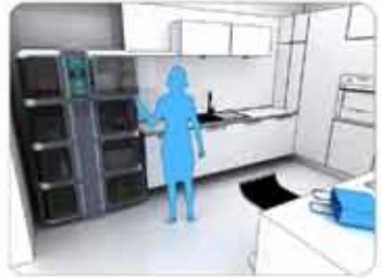
With the help of the speech recognition system, the user opens the cover of the dairy product box and the user places milk bottles into this box.
