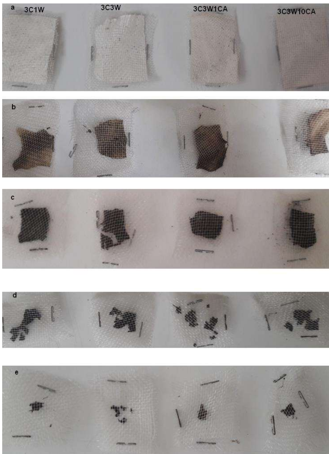
Figure 3.6 Biodegradability of films at the (a) beginning, (b) 5th day, (c) 10th day, (d) 15th day, (e) and 20th day; order of the samples in each row: 3C1W, 3C3W, 3C3W1CA, and 3C3W10CA
