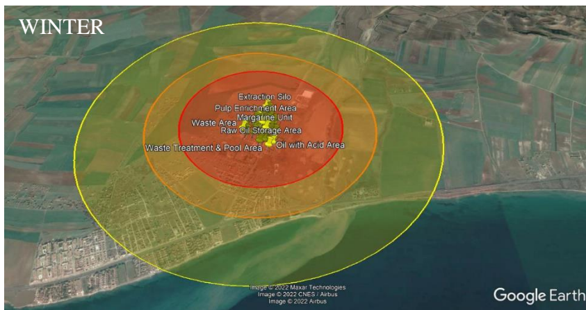
Figure 4.25. Visual representation of thermal radiation threat zone for autumn and winter with 50 % percentage of mass in the fireball on Google Earth Pro (Google Earth Pro, 2022).
