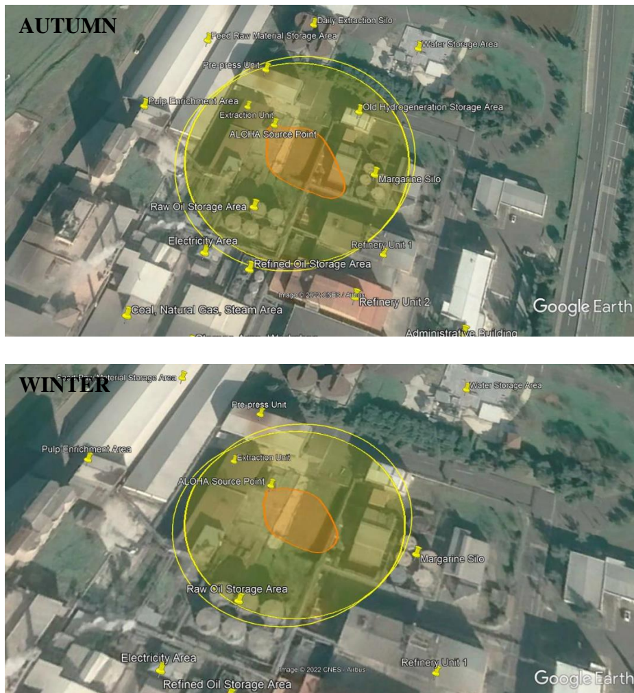
Figure 4.16. Visual representation of overpressure threat zone for autumn and winter (Google Earth Pro, 2022).
