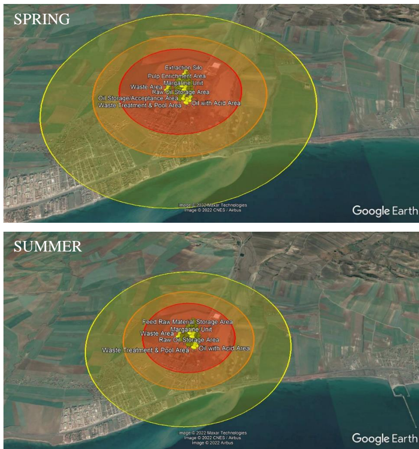
Figure 4.24. Visual representation of thermal radiation threat zone for spring and summer with 50 % percentage of mass in the fireball on Google Earth Pro (Google Earth Pro, 2022).
