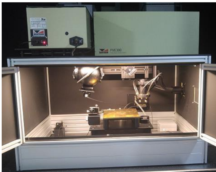
Figure 4.13. Bentham PVE300 Photovoltaic EQE (IPCE) is used for reflection/transmission measurements.
