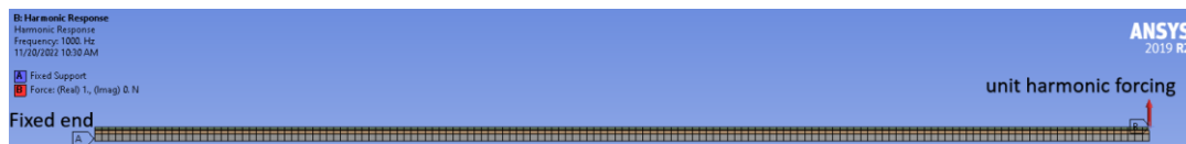
Figure 3.14. The Fixed-Free Beam Configuration
