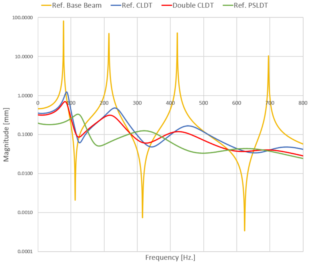
Figure 4.2. The FRF Comparison Plot between Reference Baseline Configurations
