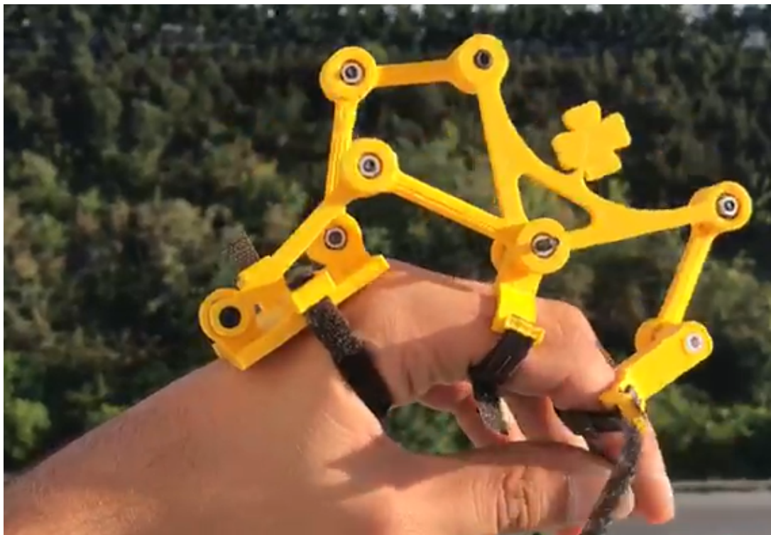
Figure 5.4: Manufactured Fully-Actuated Prototype 1 View 1
