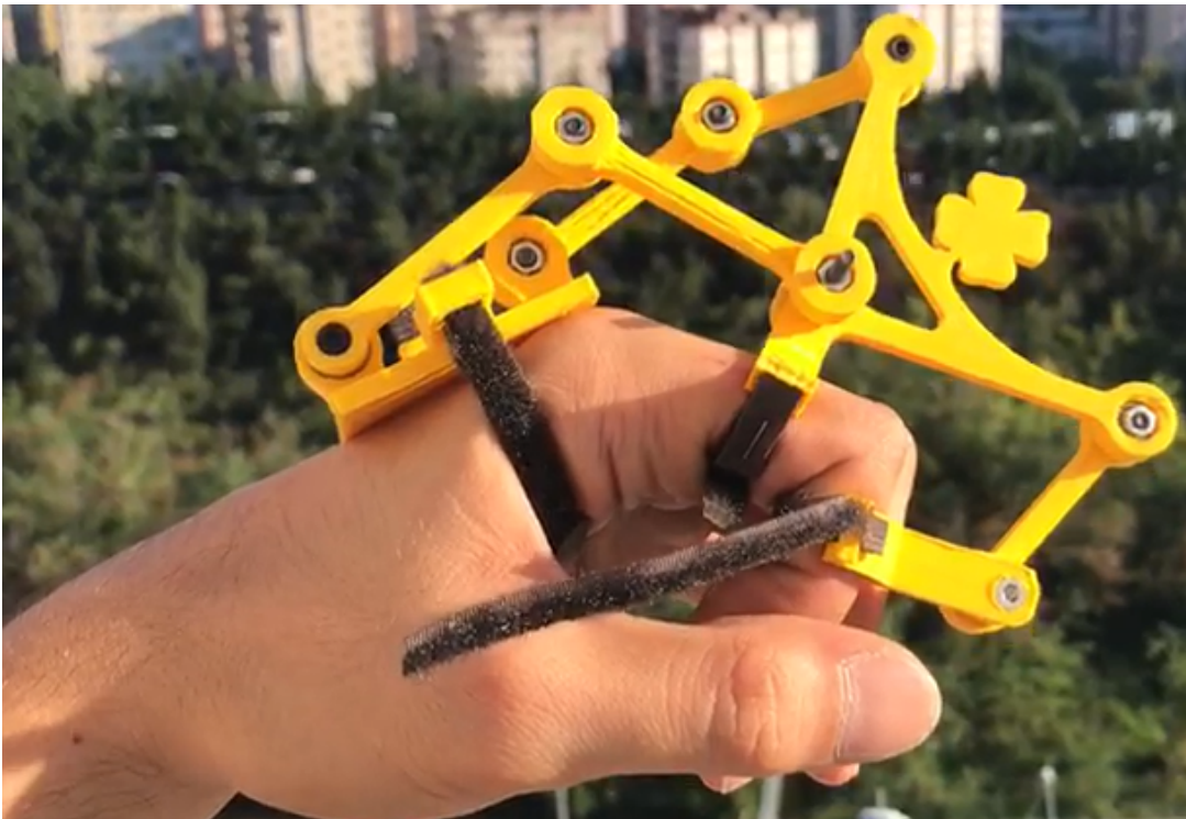
Figure 5.5: Manufactured Fully-Actuated Prototype 1 View 2
