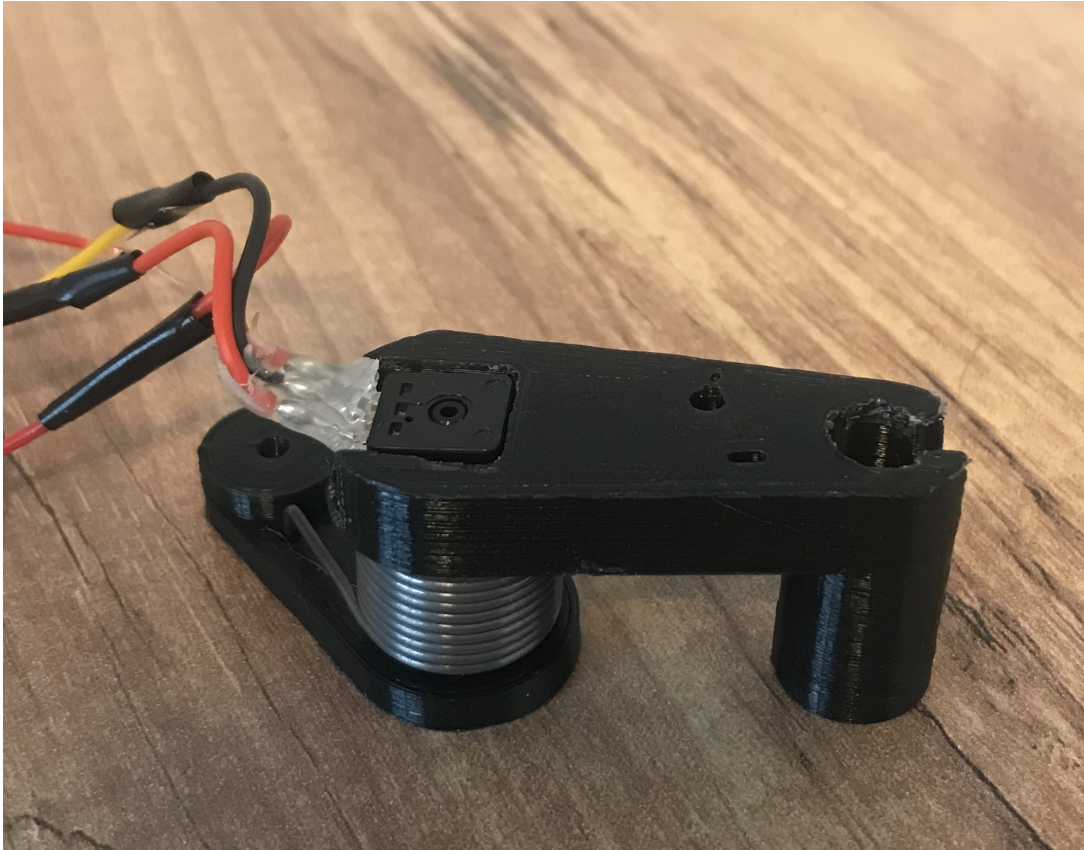
Figure 5.14: Under-actuated Adaptor View 1
