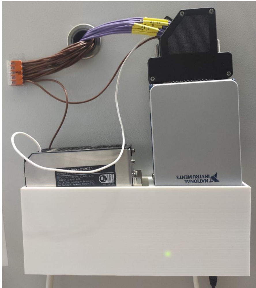
Figure 3.4 Pressure data acquisition system powered by National Instruments
