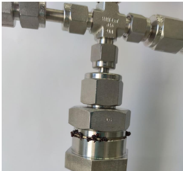
Figure 4.6 Leak through MPV body and PMRS connection occurred during with the PTFE-04 tube storage
