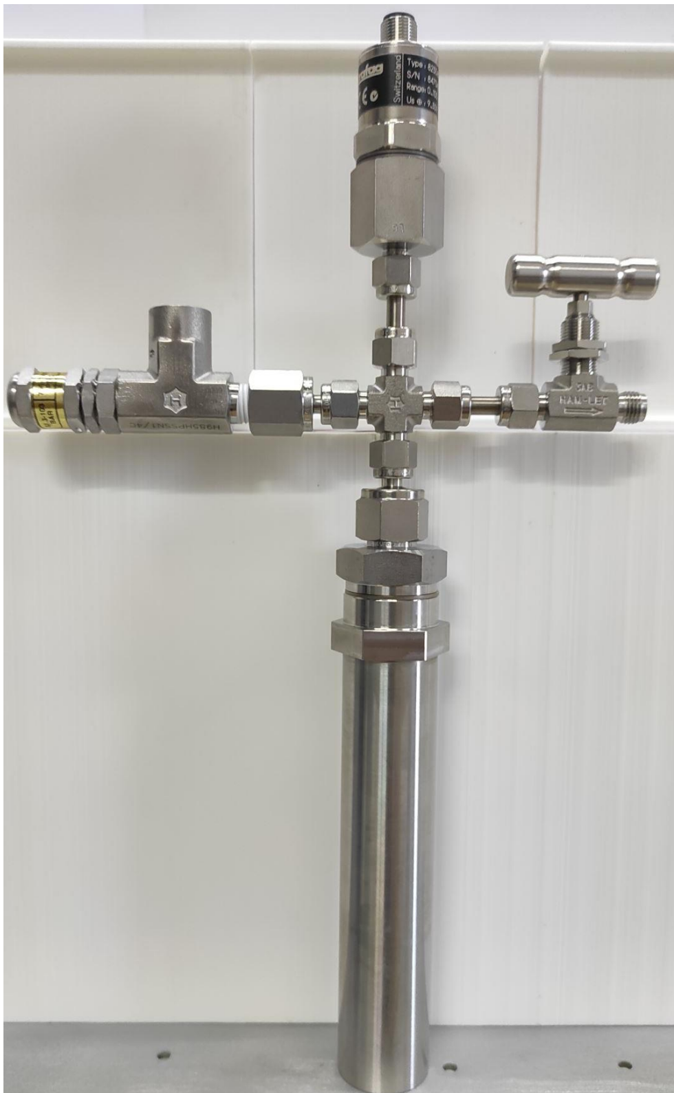
Figure 3.3 Mini Pressure Vessel Body with Pressure Measurement and Relief System (PMRS) attached (whole unit is MPV fixture) (see Table B.1 for detail)
