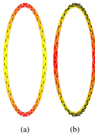
Figure 4.27: Modal currents on the elliptic ring element, illuminated by an x -polarized plane wave at 8 GHz. (a) Mode 1. (b) Mode 2.
