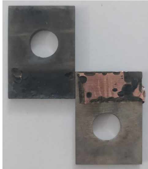
Figure 4.11 Two pieces of Al received after the brazing test performed by using copper foil as brazing filler metal
