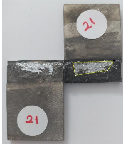
Figure 4.12 Brazed region of sample number 21
