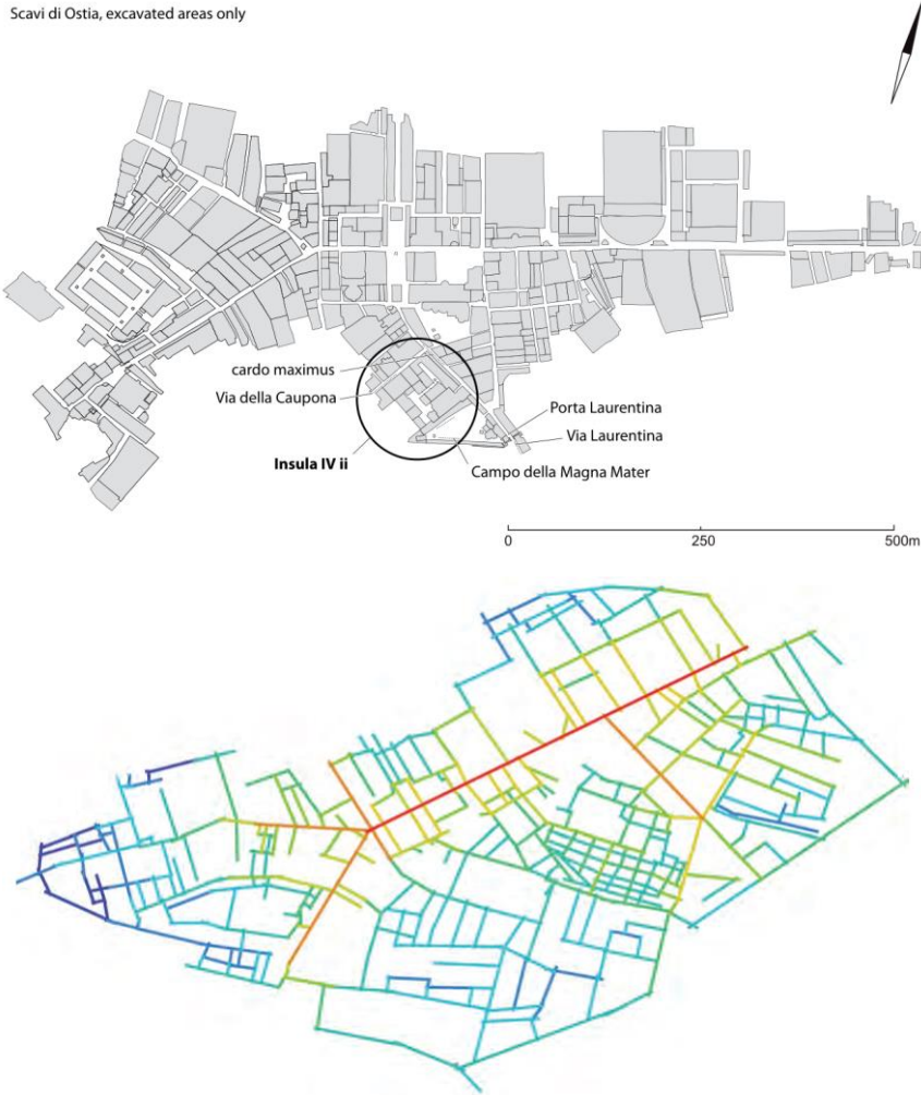
Figure 23: A map showing Ostia urban layout with the excavated areas and insula iv (top), a global axial integration graph (bottom) for the Ostia street network (Stöger, 2011, p. 214)
