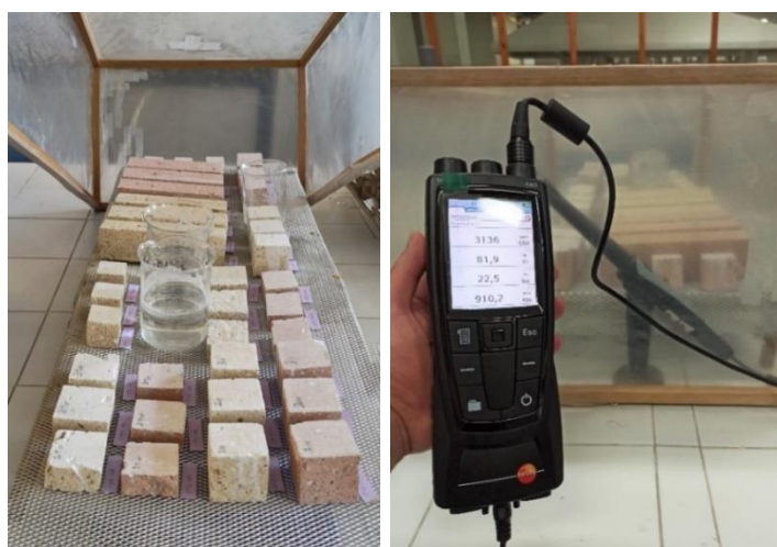
Figure 3.7. Carbonation process of CYT and CPT samples in a climate chamber containing 88% high relative humidity and enhanced carbon dioxide conditions (left), the TESTO 480 indoor air quality measuring device monitored and recorded changes in RH, temperature, and CO 2 concentrations.
