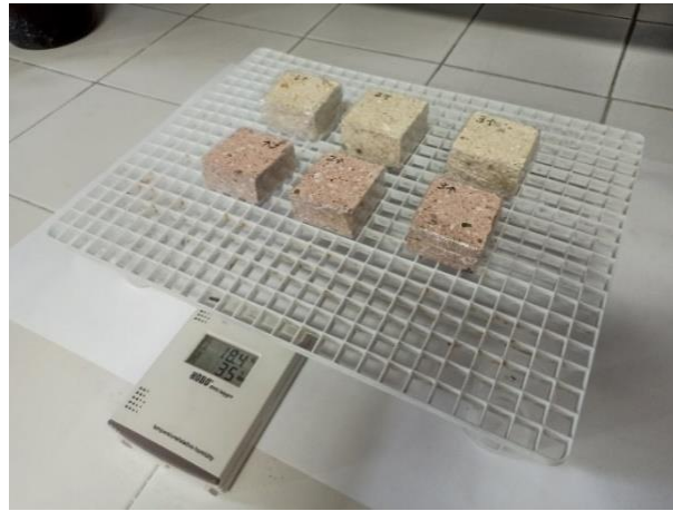
Figure 3.13. CYT and CPT samples left on a grid sheet for drying at constant atmospheric conditions of 20^{\circ}\text{C}\pm 2 and 30\%\pm 5 RH.
