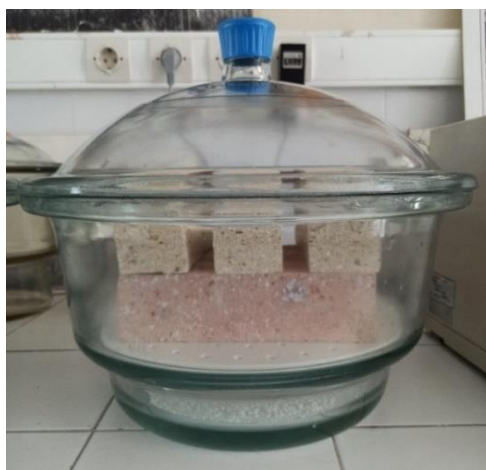
Figure 3.17. CYT and CPT samples placed in a desiccator filled with granular calcium chloride to control the humidity level in the chamber.
