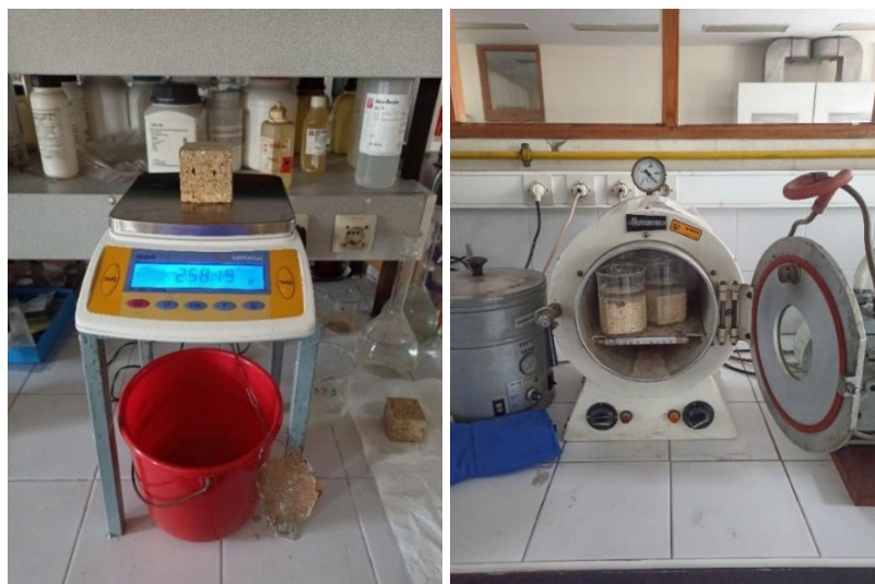
Figure 3.9. Measurement of sample weights after 24 hours saturation with distilled water (left), samples being completely water-saturated in the HERAEUS vacuum chamber at 0.132atm (100 torr) pressure.
