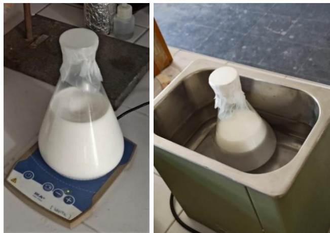
Figure 3.4. Nano dispersive calcium hydroxide solution magnetically stirred for 24 hours (left), ultrasonic vibration of the solution for 3 hours (right).
