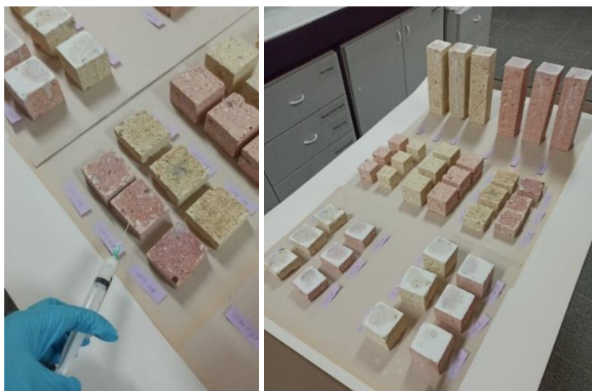
Figure 3.6. The process of applying a nano dispersive calcium hydroxide solution to the surfaces of fresh CYT and CPT samples of various sizes by capillary suction (left), the treated tuff samples left to dry under laboratory conditions (40±5% RH) for 24 hours.
