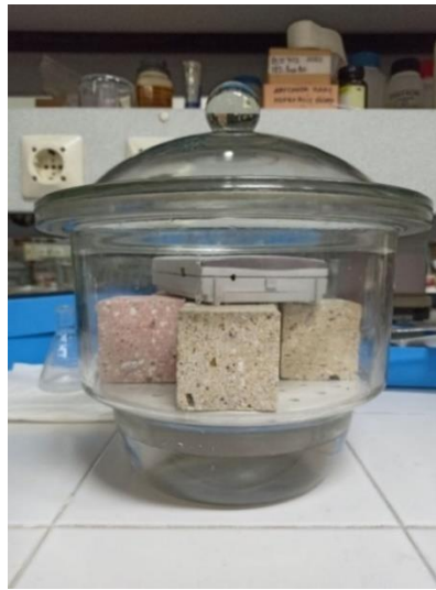
Figure 3.10. CYT and CPT samples kept under high relative humidity conditions in a desiccator.
