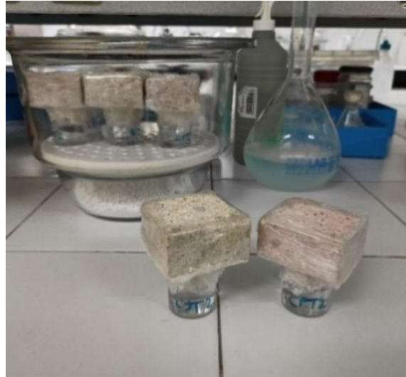
Figure 3.11. CYT and CPT test samples assembled into the containers prepared for the water vapor permeability tests.
