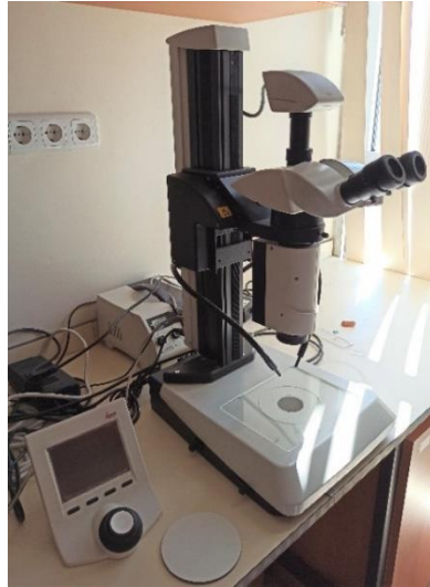
Figure 3.21. Leica Stereo Optical Microscope in the laboratory utilized for analyzing microstructural properties of materials through stereomicroscopic images.
