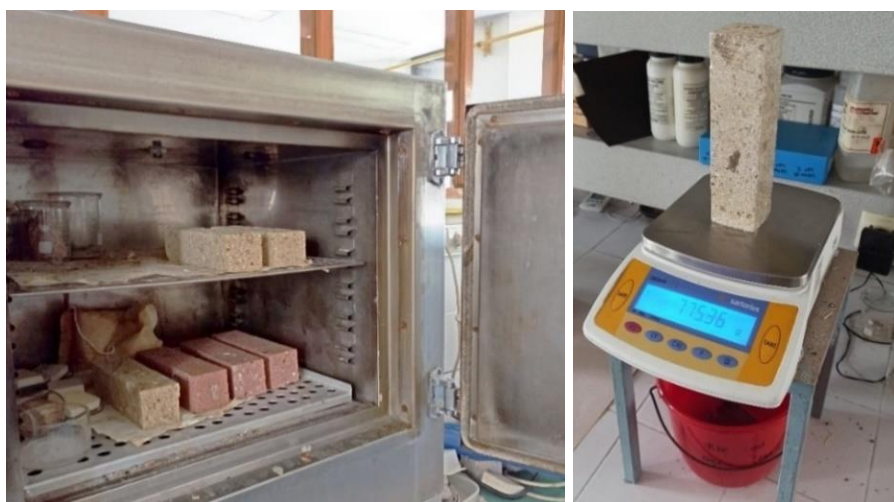
Figure 3.14. CYT and CPT samples with the dimension of 5x5x20 cm dried in the oven at 60°C to a constant weight (left), weighing the dry sample of CYT covered with a stretch film were (right).
