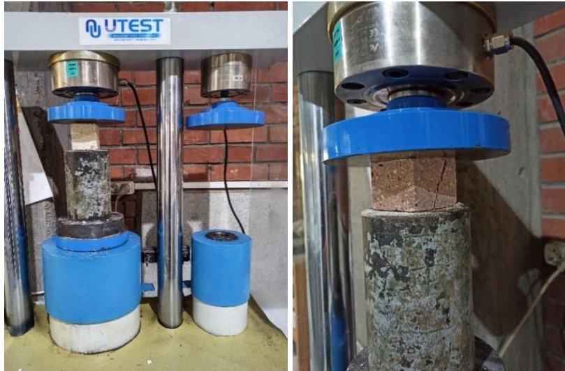
Figure 3.19. Cappadocian Yellow Tuff in compressive strength test setup (left), Cappadocian Pink Tuff in the compressive strength test setup and the crack formed on the sample (right).
