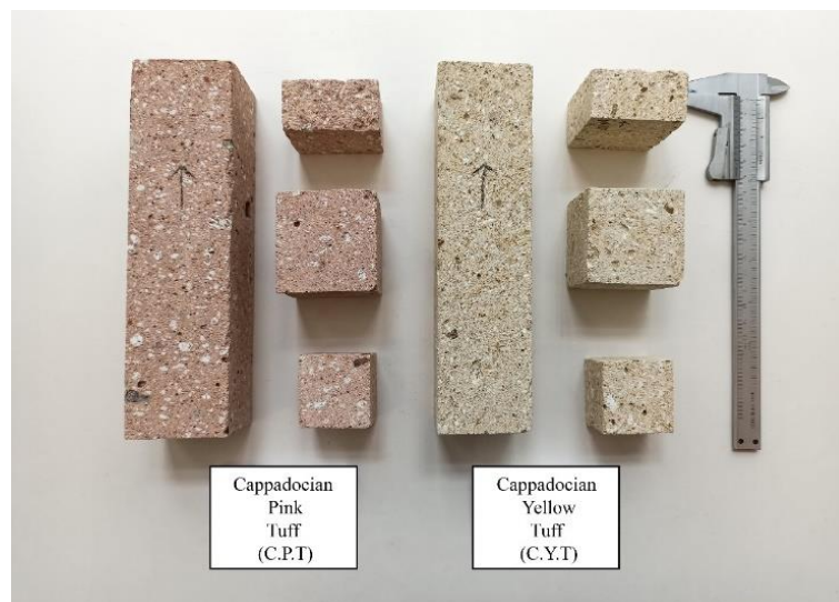
Figure 3.3. Tuff samples prepared for the laboratory tests with the dimensions of 5×5×5 cm, 5×2.5×5 cm, 5×5×20 cm, 4×4×4 cm.
