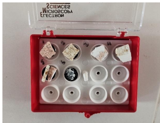
Figure 3.22. Small pieces of both fresh and treated CYT and CPT tuff samples and powdered nano dispersive \text{Ca}(\text{OH})_2 solution located in the stubs prepared for the SEM and EDAX analyses.
