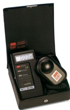
Figure 3.10 Lux meter RO1335 by Rotronic to measure illuminance in the METU cafeteria dining halls
