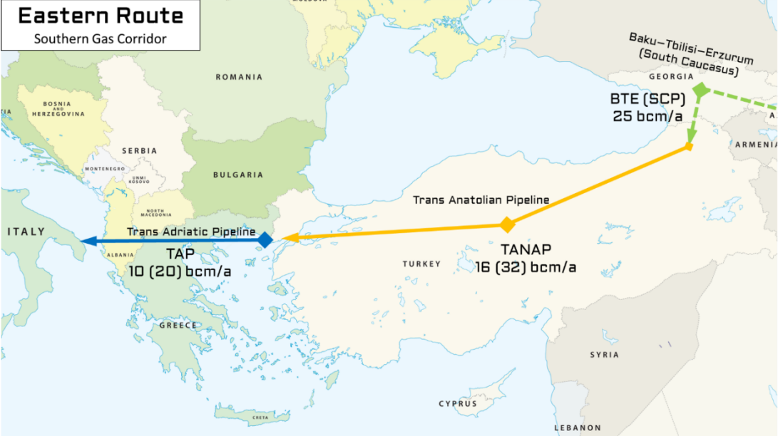
Figure 3.14: Simplified Pipeline Connections to the EU from Caucasia (with Potential Increase in Capacity)
