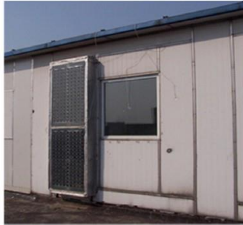
Figure 2.13 PV Trombe Wall, a hot box constructed on the roof-top of an office building located at 37.86 N latitude (Sun et al., 2011)
