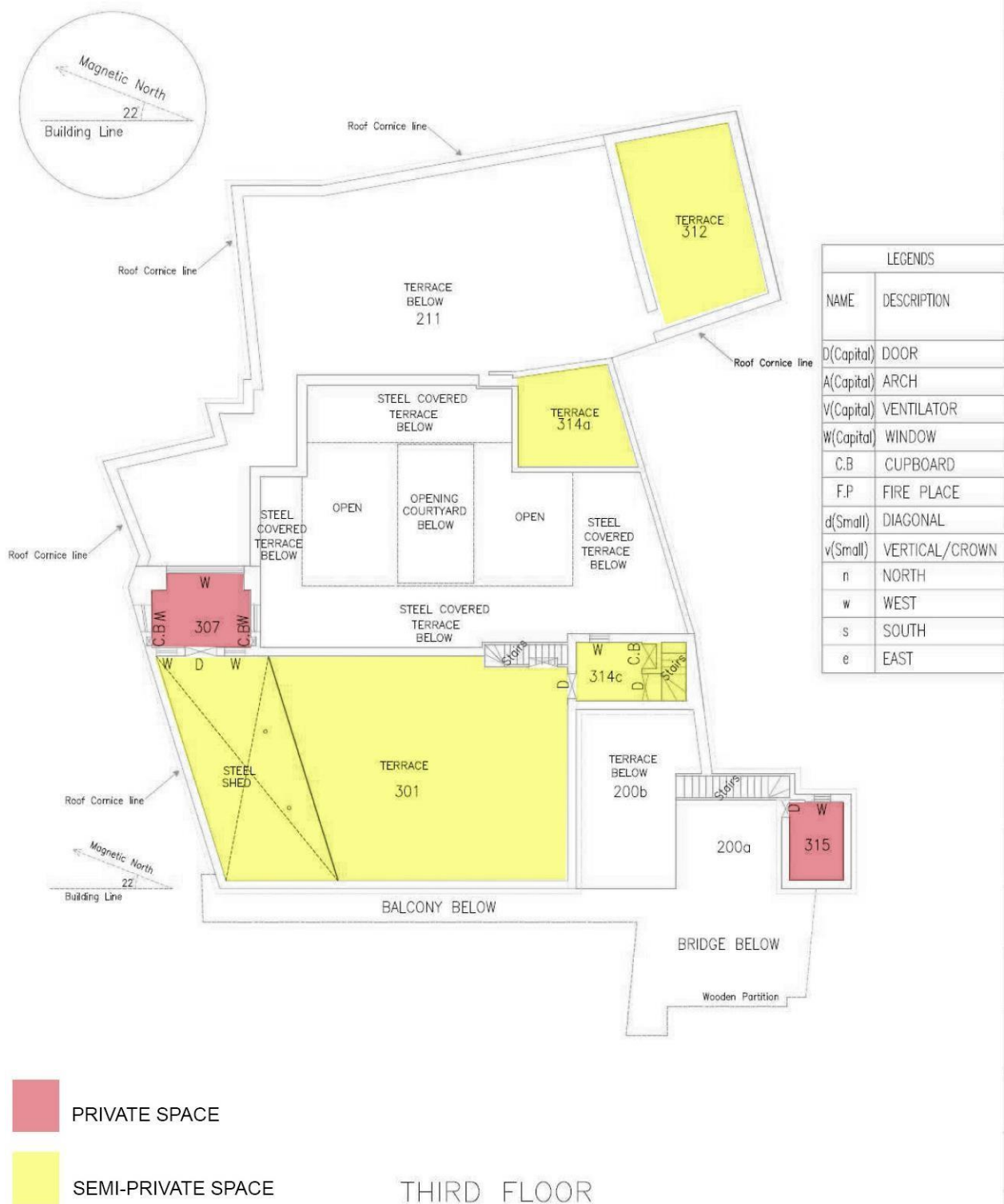
Figure 32: Third Floor Plan Public Private spaces. (Adopted: Rogers Kolachi Khan & Associates (Ltd.), Assessment of the Existing Condition at the Historic Haveli Sujan Singh, Rawalpindi, Pakistan. )
