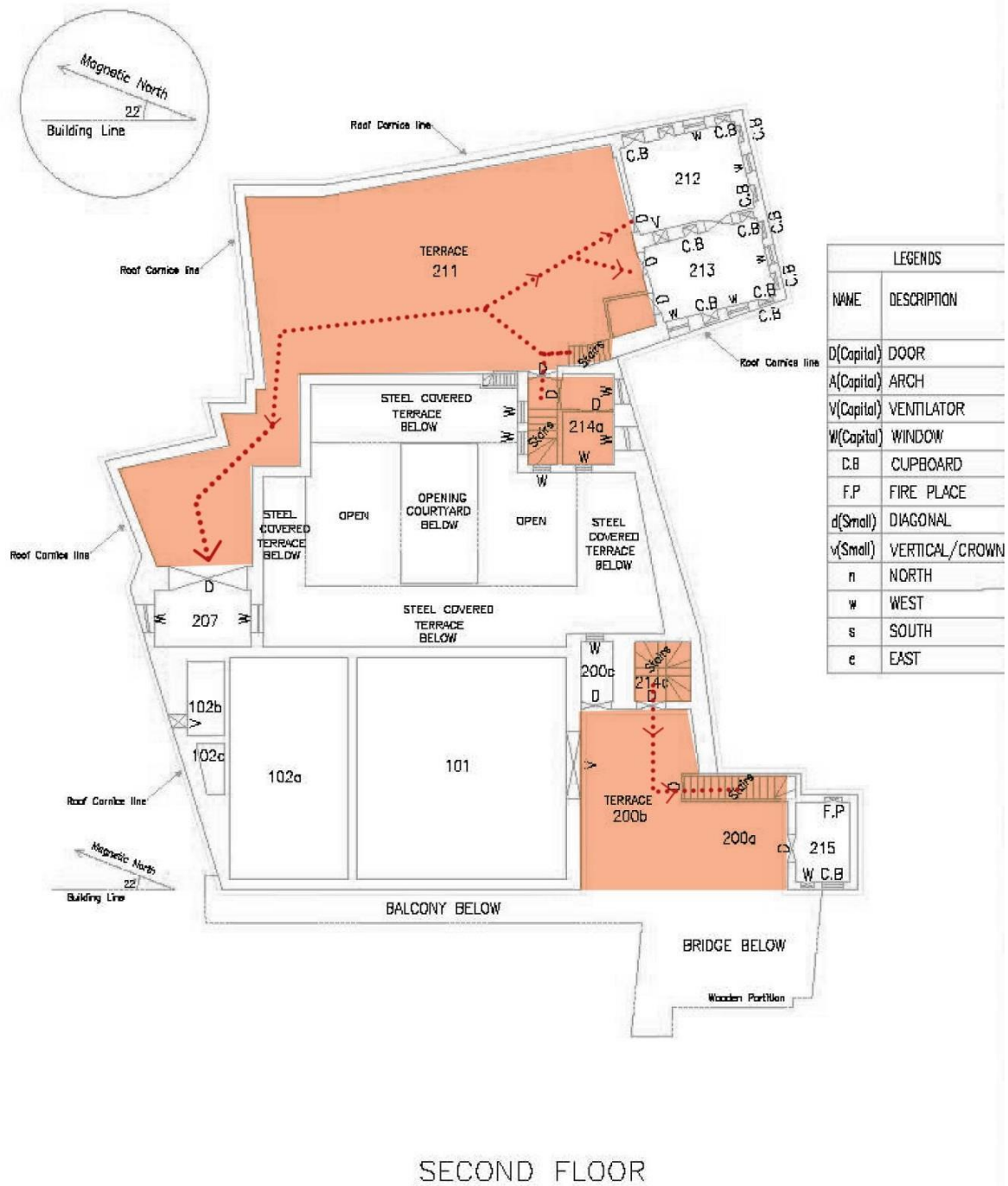
Figure 99: Circulation and Route plan of the Second Floor. (Adopted: Rogers Kolachi Khan & Associates (Ltd.), Assessment of the Existing Condition at the Historic Haveli Sujan Singh, Rawalpindi, Pakistan. )
