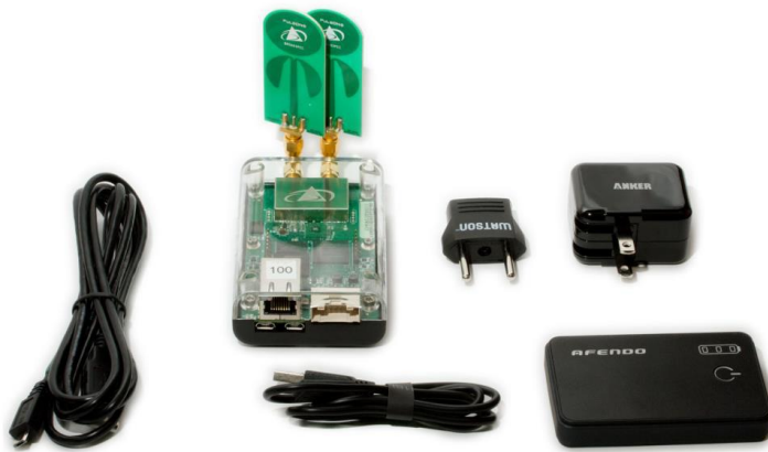
Figure E.1. TimeDomain PulsON 440 Radar Kit [31]
