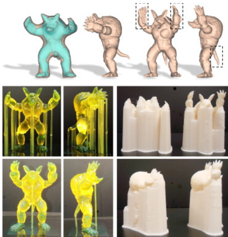
Figure 2.6: Support volume reduction by modification [15]
