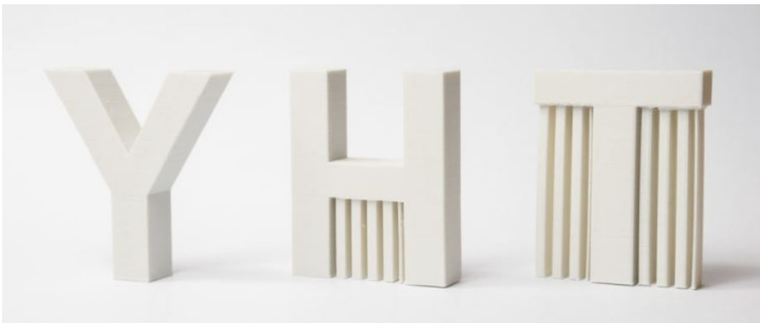
Figure 2.2: Sample Cases for Overhanging and Bridging Support Requirements [7].
