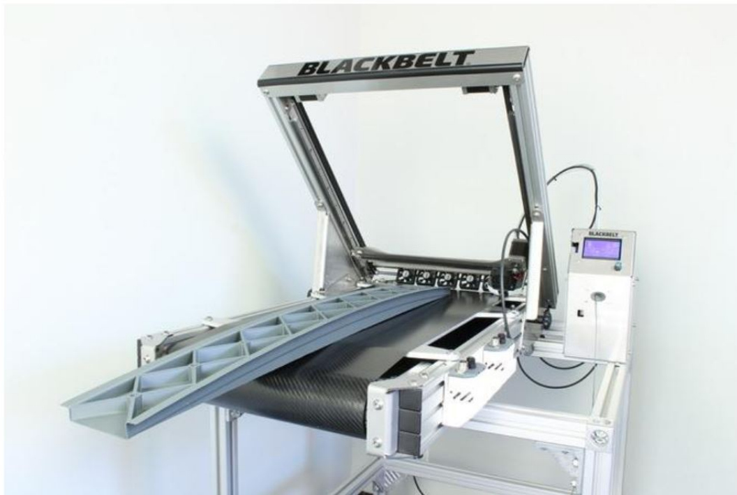
Figure 2.12: Inclined 3D printer with a conveyor belt, BlackBelt 3D [27]
