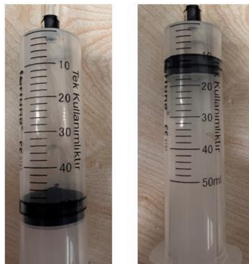
Figure 3.8 The injector used to pump water
