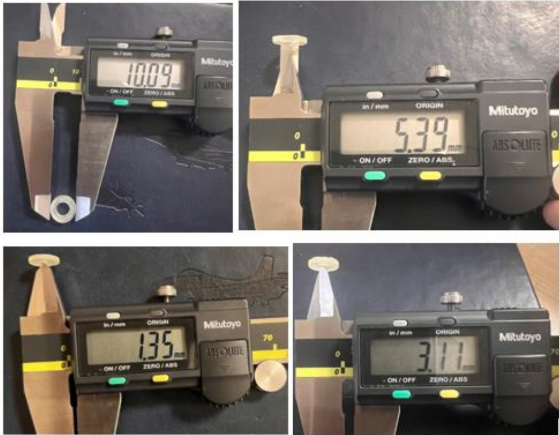
Figure 3.4 99%, 90%, and 70% occlusion sample diameter
