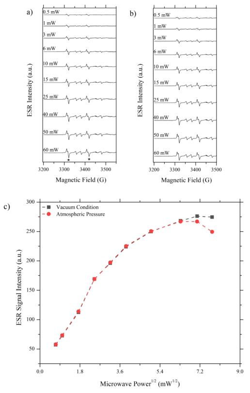
**Figure 4.** Saturation-recovery CW-ESR Experiment **a)** Mn(II)/Plasticine in vacuum condition **b)** Mn(II)/ plasticine in atmospheric pressure **c)** Signal intensity vs. microwave power<sup>1/2</sup> analysis for atmosphere exposed and evacuated Mn(II)/plasticine.
