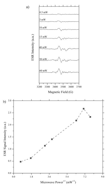
**Figure 5.** Saturation-recovery CW-ESR experimental results for  $0.5\% Pd/TiO_2$  **a)** Spectrum **b)** Signal intensity vs microwave power<sup>1/2</sup> analysis.
