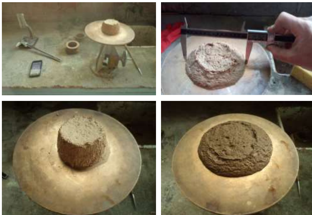
Figure 3-5: Set-up to determine the consistency of fresh mortars (flow table test)
