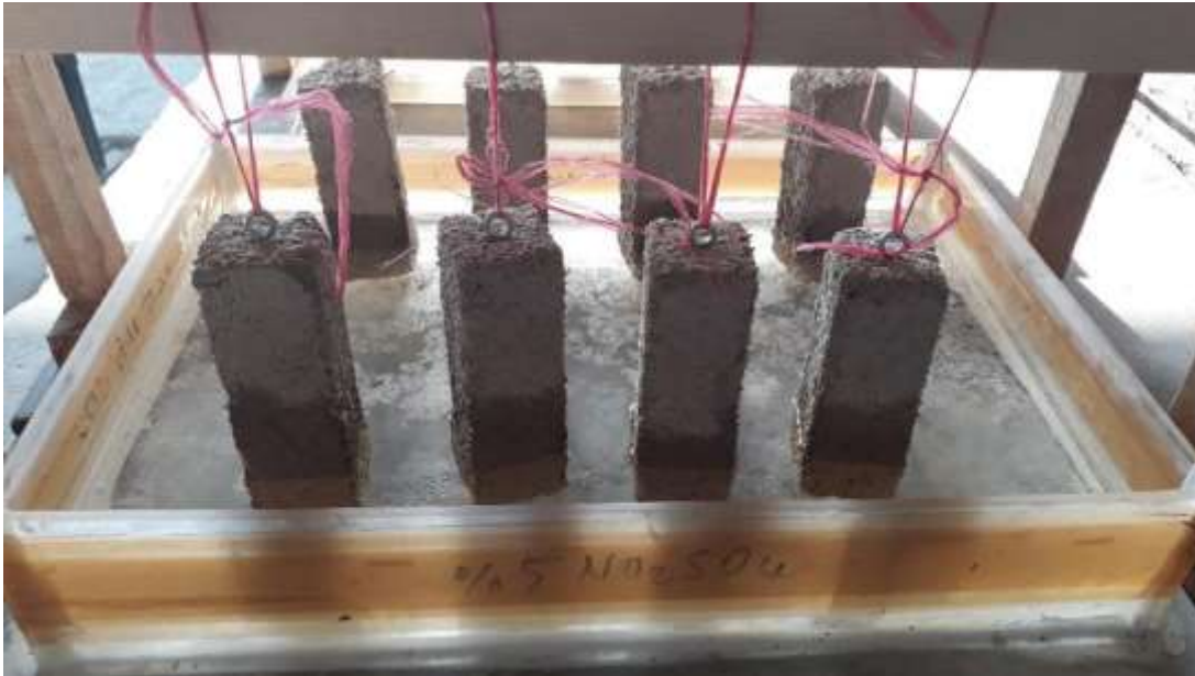
Figure 3-11: Set-up for measuring the water resistance of samples – The length of the strings was calculated for the samples to be hung 4cm in water
