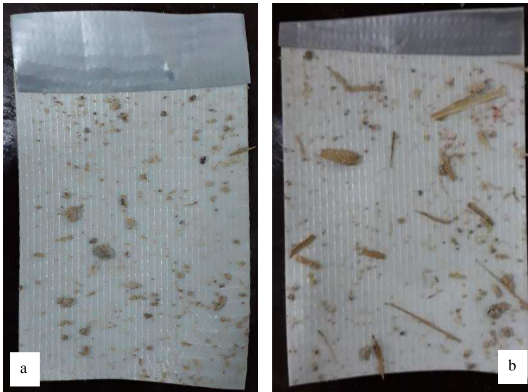
Figure 5-20: Difference of type of particles attached to the band accounting for the weight difference even if the number of particles is similar. a) samples reinforced with a large amount of sand and few fibres. b) mortars reinforced with a large amount of fibres but few sand.
