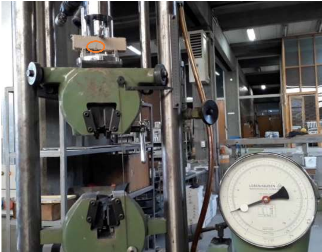
Figure 5-17: Conservation of the strength of the mortar reinforced with chaff despite the appearance of cracks on the surface of the specimen (circled on the picture)
