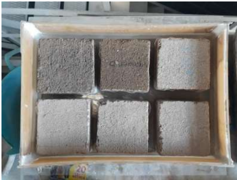
Figure 3-13: Samples placed in a waterproof container to determine the water capillarity absorption
