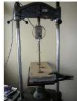
Figure 2-13: Adhesive strength pull-out device (Deliniere et al., 2014) (The standard procedure corresponds to the plaster directly applied on a concrete panel whereas the modified procedure consists in applying a clay slip on the concrete panel before applying the plaster)
