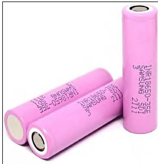
Figure 2.2. Cylindrical cells of Samsung company. Samsung 35E is the name, 18650 is cell type, 3500 mAh is capacity(energy), and 8A is the maximum continuous power rating. INR abbreviation stands for NMC type cathode chemistry.[3]
