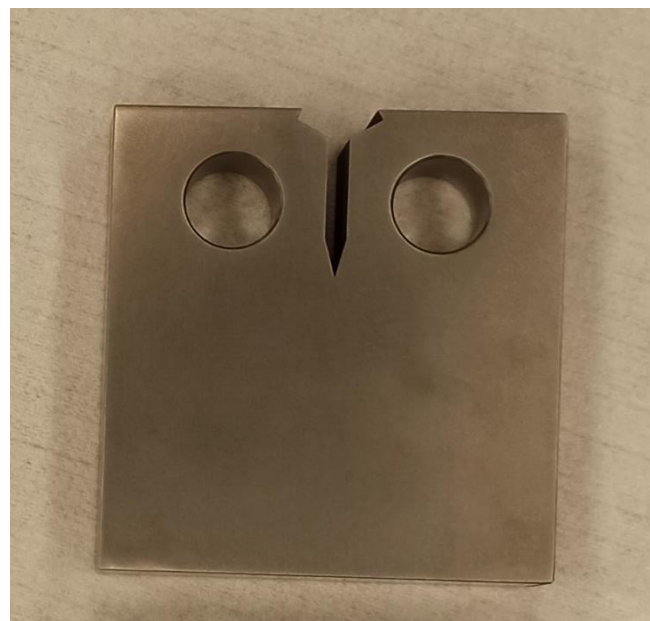
Figure 3-12. Finished CT (50) test specimens
