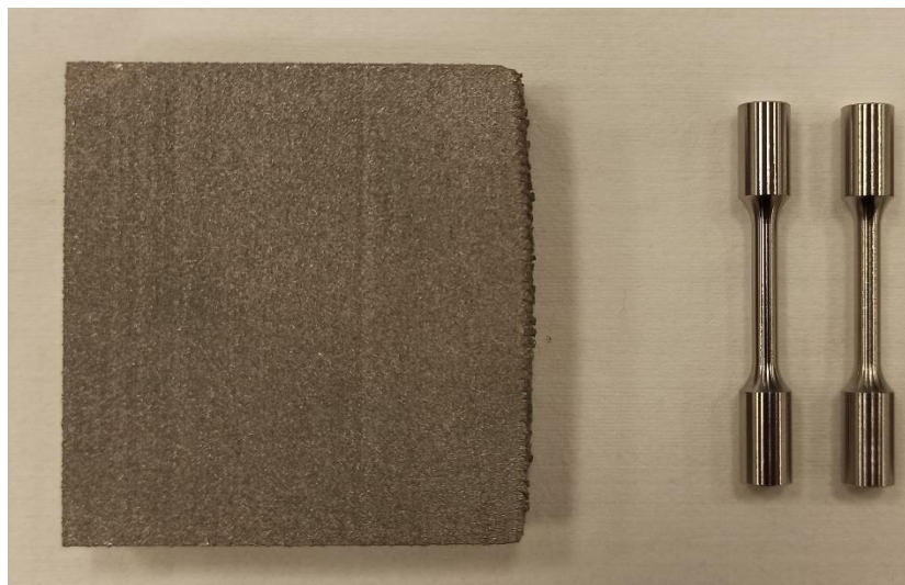
Figure 3-8. Block fabricated by EBM and finished tension test specimens
