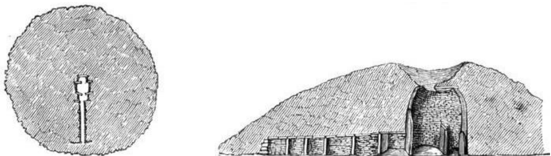
Figure 51. Ground plan and section of chambered cairn with a corbelled roof at Camster
