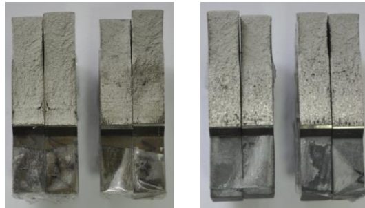
Figure 88. Fracture surface of 200 and 200H
