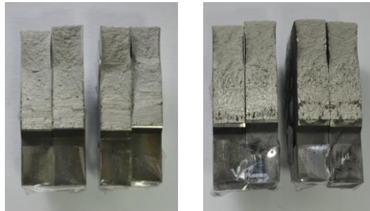
Figure 87. Fracture surface of 200 and 200H
