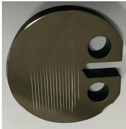
Figure 22. Fatigue crack growth sample and drawn lines
