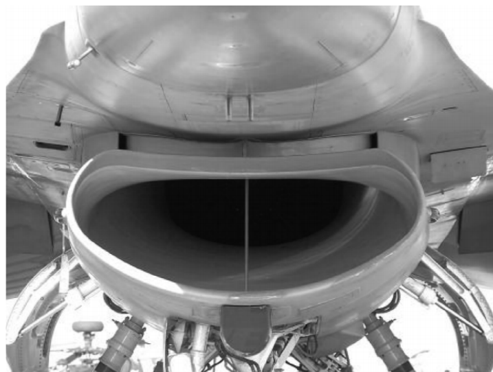
Figure 1.3: Boundary Layer Diverter on the General Dynamics/Lockheed Martin F-16BM [1]
