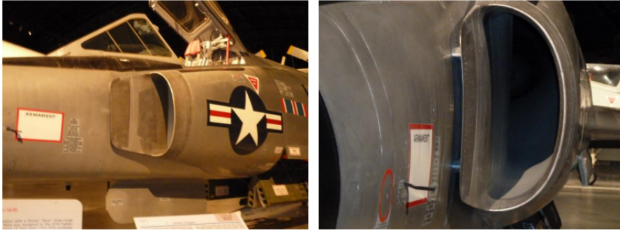
Figure 1.4: Splitter Plate on F-102 [4]
