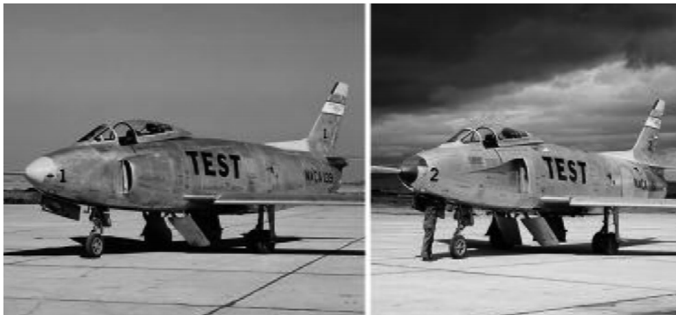
Figure 1.2: Early Examples of Air Integrated Inlet Designs on YF-93A research aircraft(from left to right): Scoop and Naca Flush Intake), Taken From Reference [1]
