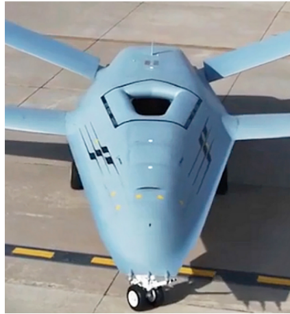
Figure 1.6: Diverterless Intake on MQ-25
