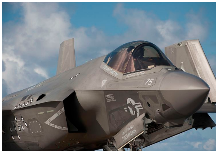
Figure 1.5: Diverterless Intake on F-35
