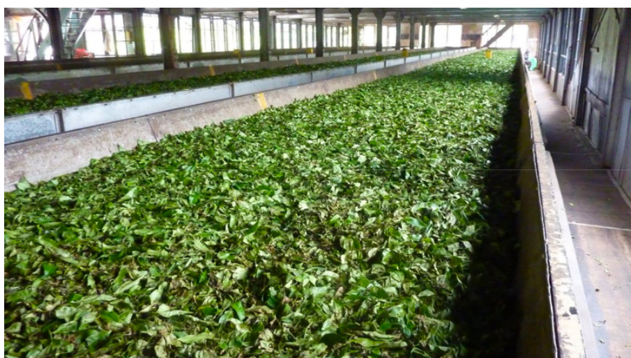
Figure 5.17. Withering Process in Tea Factory ( Orçay, n.d. )
