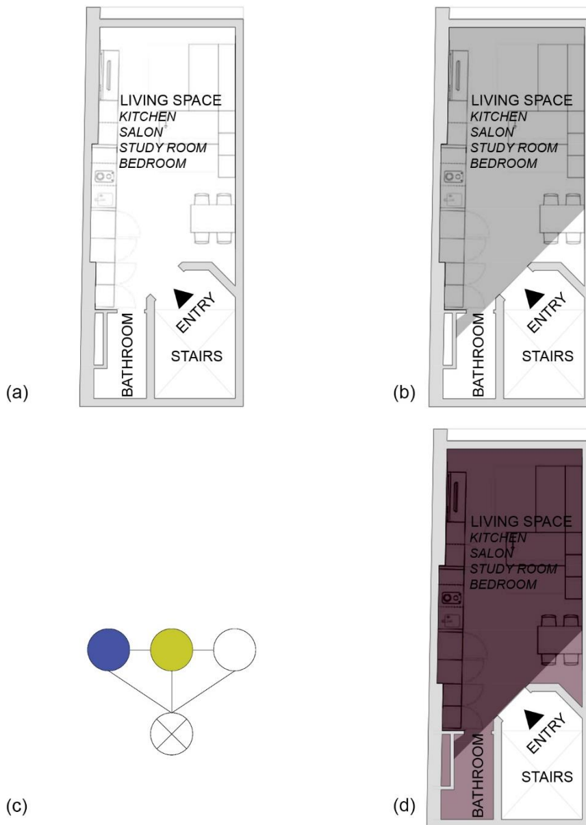
Figure 5.28. (a) Plan of Microloft Yarasa , İstanbul, 2011 (redrawn by the author) 304 , (b) Visual accessibility from the entrance diagram; (c) Spatial relationship, accessibility and stratification diagram; (d) Spatial separation diagram
