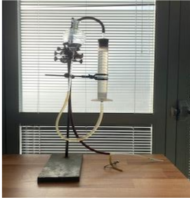
Figure 3.1. Water displacement device used for the measurement of total biogas production
