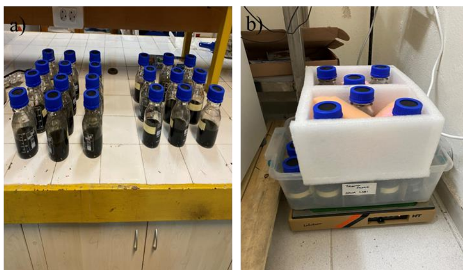
Figure 3.10. a) The reactors filled with inoculum and cattle manure and b) the reactors on the shaker in Set 2
