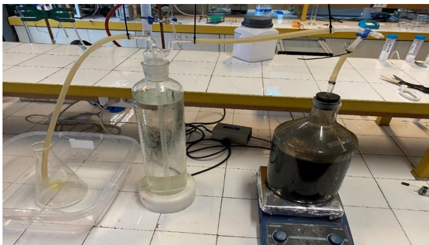
Figure 3.12. The reactor set-up for acclimation of inoculum
