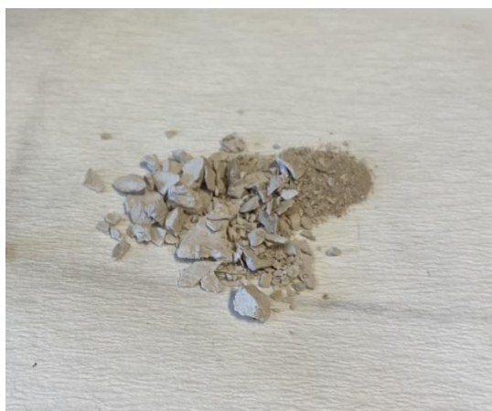
Figure 3.14. Precipitate scratched from the filter paper to be analyzed with XRD
