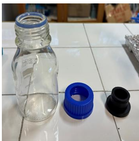
Figure 3.6. The serum bottle, cap and stopper used in Set 2, Set 3 and Set 4
