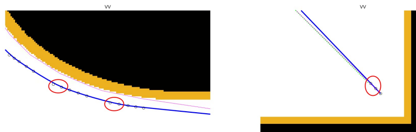
Figure 3.11: Generated helper control points at end point
