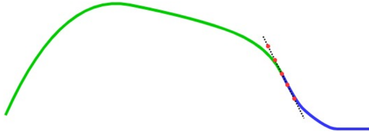
Figure 3.2: Concatenated Bezier curves with collinear control points.
