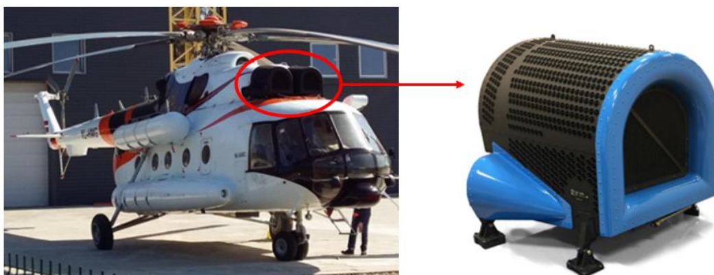
Figure 2.2. Mi-8/17 helicopter intake Vortex tube system. [6, 7]
