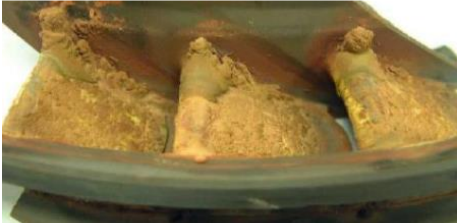
Figure 1.4. Molten impurities on turbine blades. [4]
