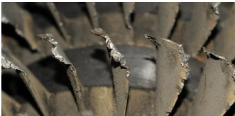
Figure 1.3. Damaged compressor blades. [3]
