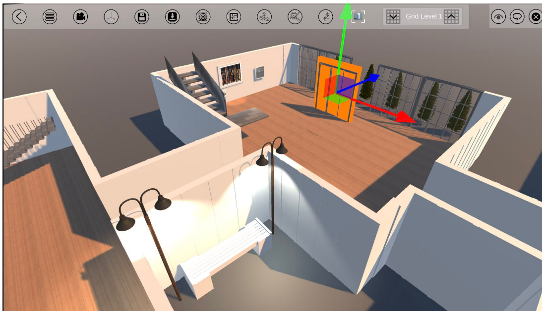
Figure 7: Output of BSP Algorithm after user intervention.
