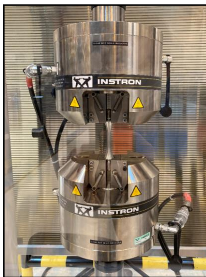
Figure 27 Instron 8801 servohydraulic test bench (performed at TAI Structural Test)
