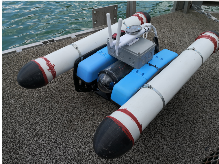
Figure 5.1: The platform used in the experiments. It consists of the main body, catamaran floaters on both sides and the communication assembly at the top.
