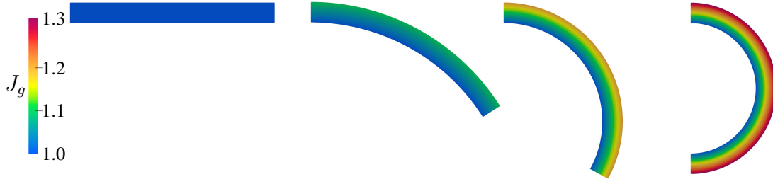
Figure 4.4: Growth-induced deformation of a 2D plate in different time increments such as t = 0 , t = 0.33 , t = 0.66 and t = 1.0 , respectively. The contour provides the variation of J_g .
