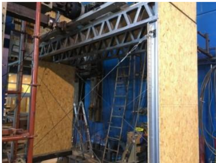
Figure 8.4 Steel cables used for out-of-plane stability
