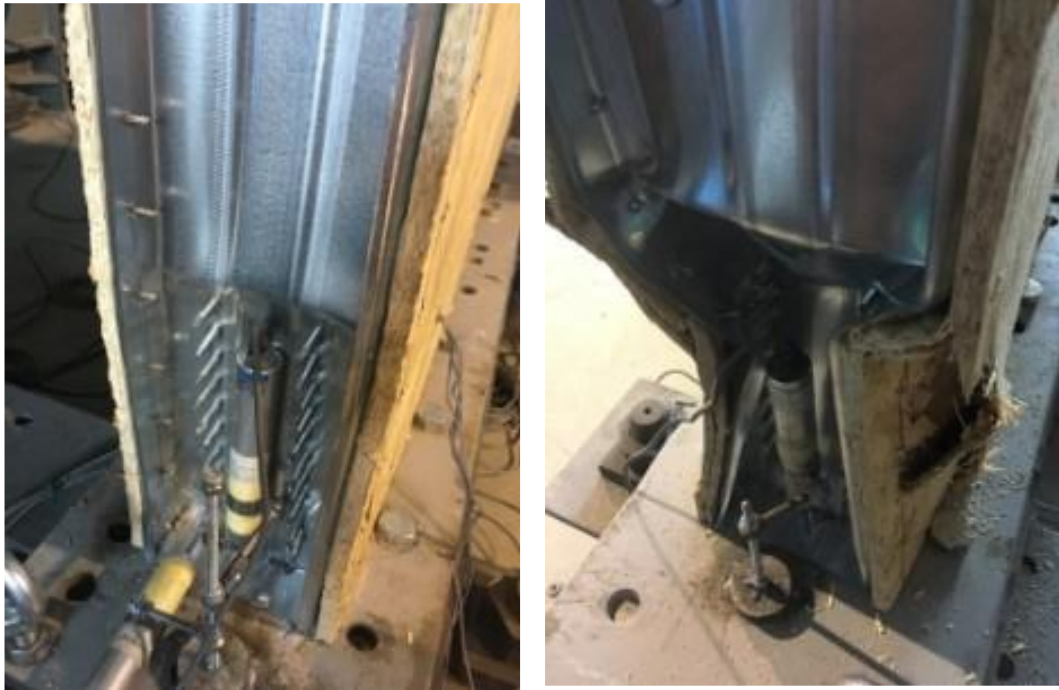
Figure 8.14 Buckling of studs observed in specimen WA-7
