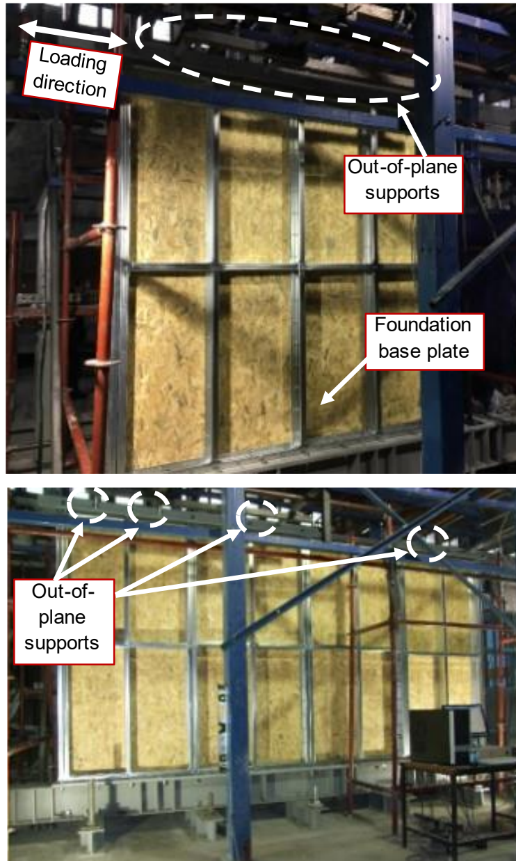
Figure 6.4 Details of wall panel test setup
