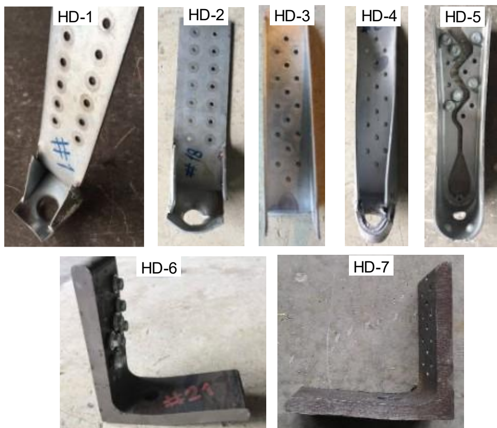
Figure 3.12 Deformations observed in hold down devices at the end of load tests
