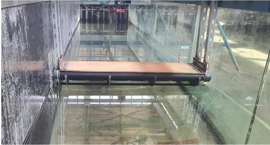
Figure 3.7: Anchored Floating Platform in Irregular Wave Flume (Frontal View)
