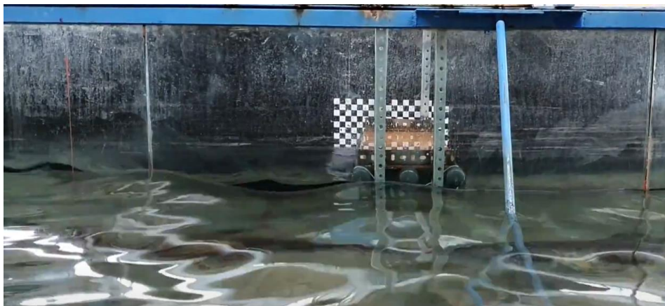
Figure 3.6: Anchored Floating Platform in Irregular Wave Flume (Side View)
