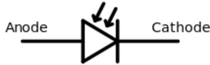
Figure 2.51. Photodiode electronic symbol
