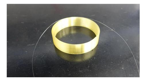
Figure 4.2. Fiber optic coil
