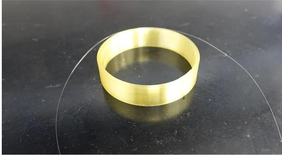
Figure 4.2. Fiber optic coil
