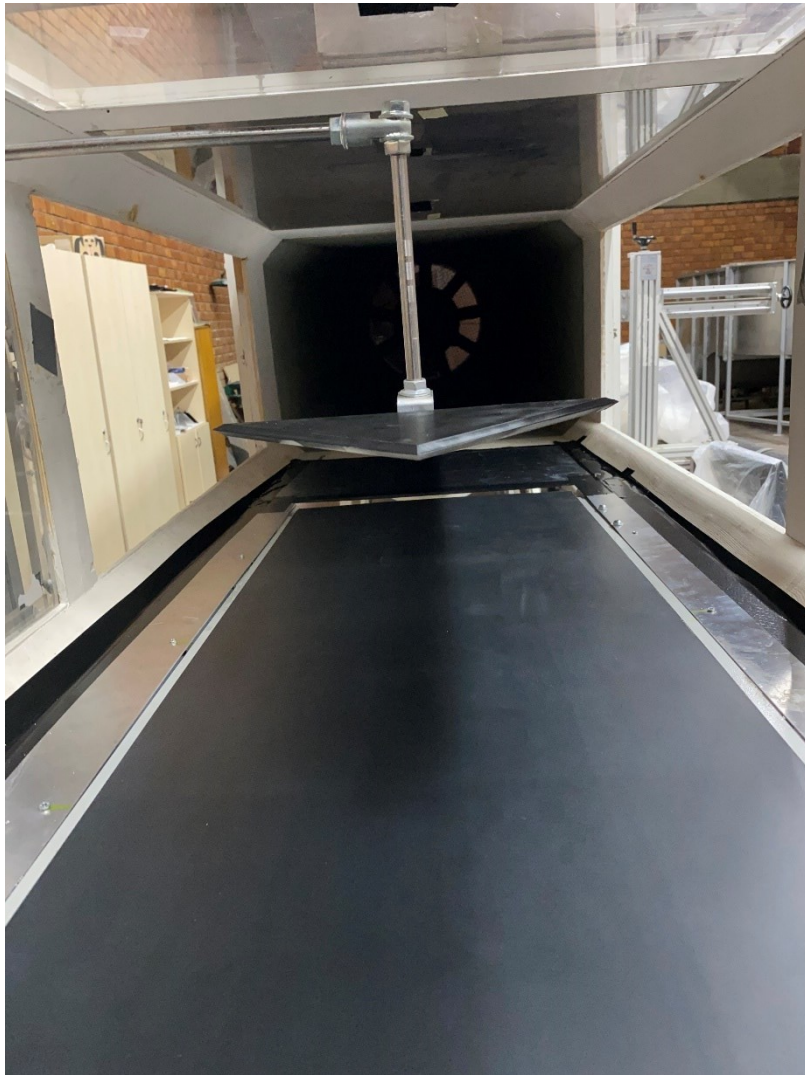
Figure D - 3 The delta wing 1a and tunnel test section with moving belt system
