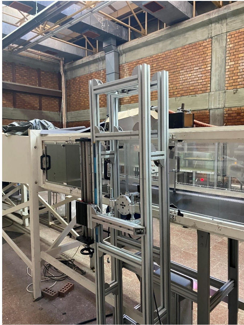
Figure D - 7 The reverse delta wing 2e, modified MPS and moving belt system
