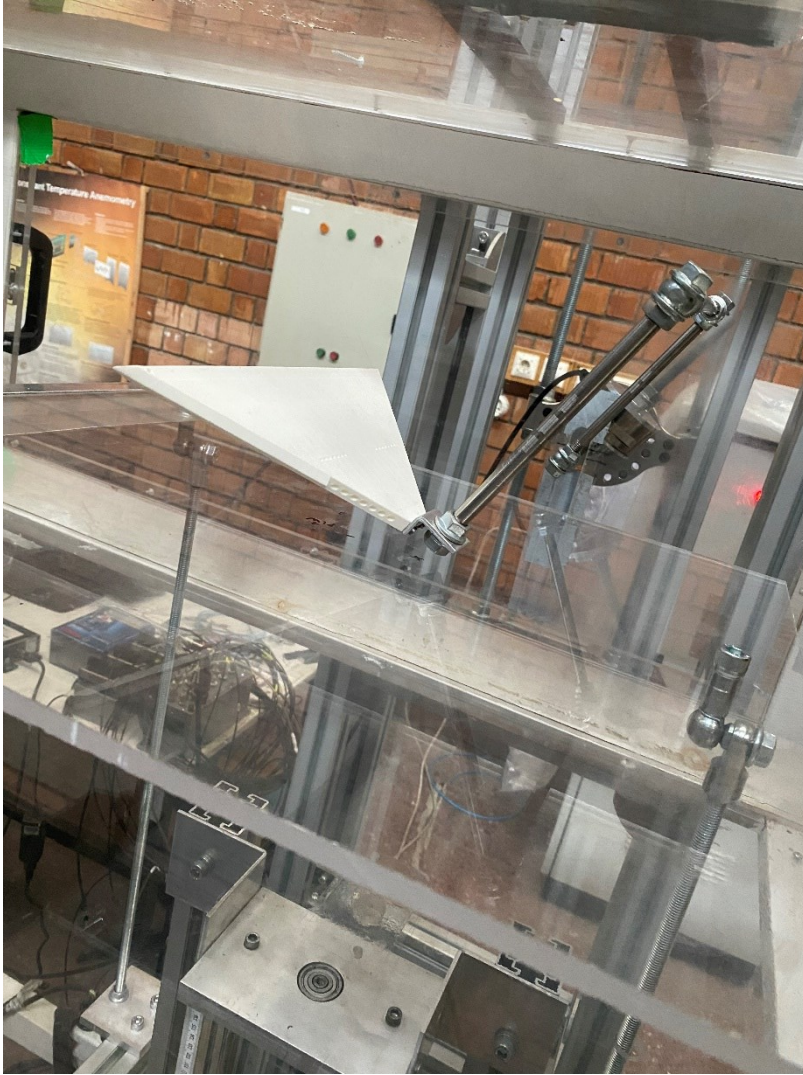
Figure D - 1 The reverse delta wing 2a in extreme ground effect for static ground condition
