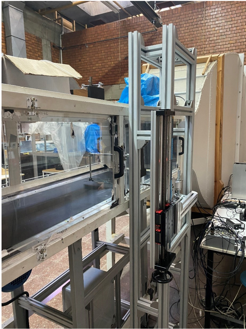
Figure D - 8 The reverse delta wing 2e, modified MPS and moving belt system
