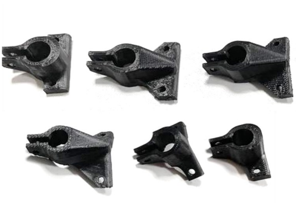
Figure B - 10 Top and perspective views of the 3D printed brackets for thin wings
