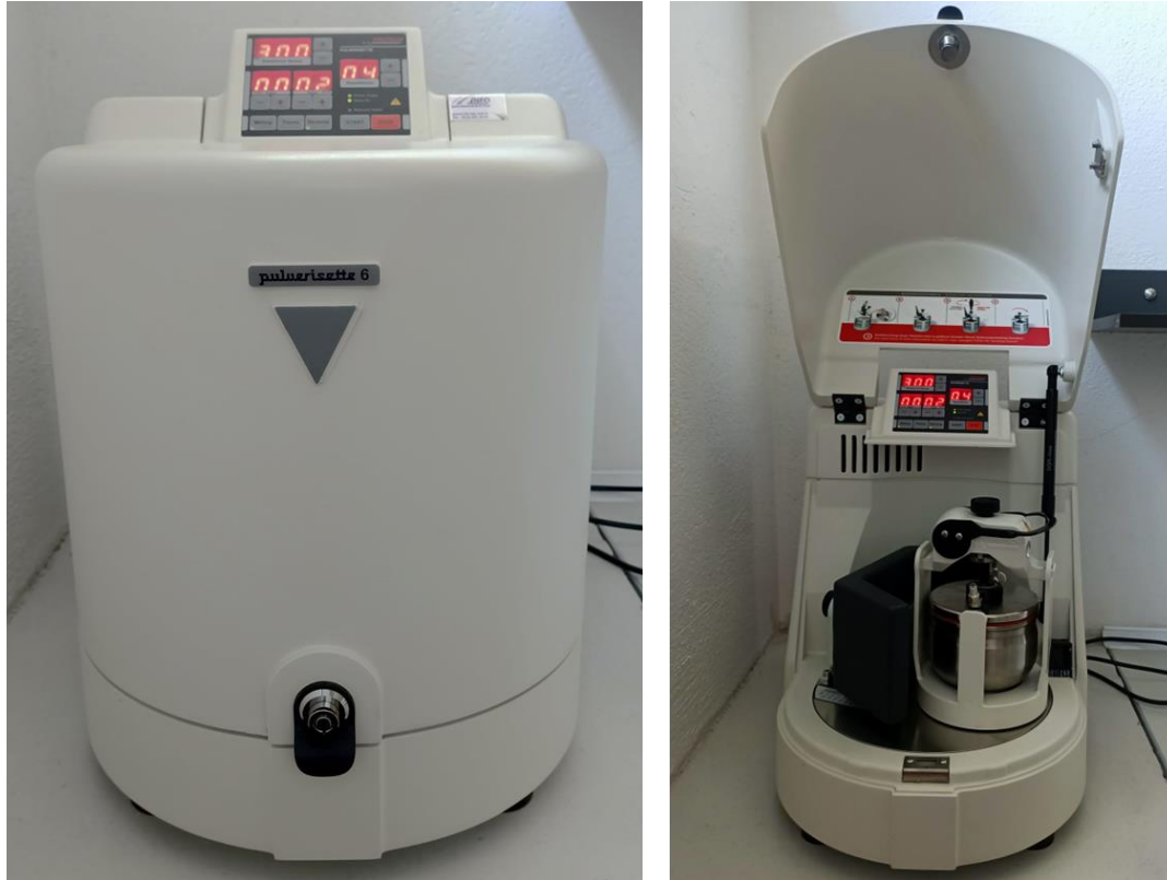
Figure 3.3. The ball mill machine setup used for mechanical mixing.
