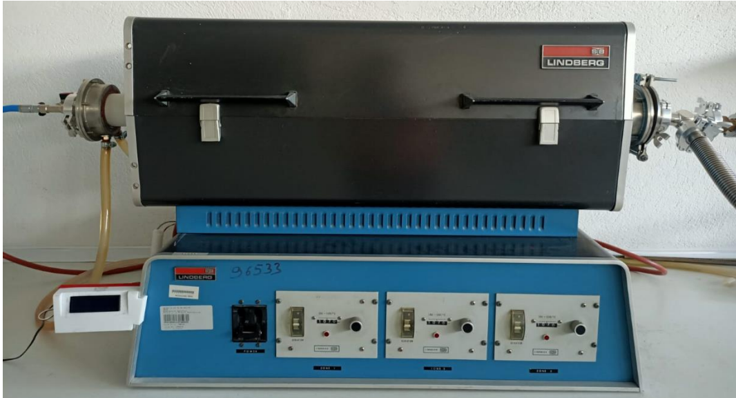
Figure 3.7. The tube furnace used for heat treatments.
