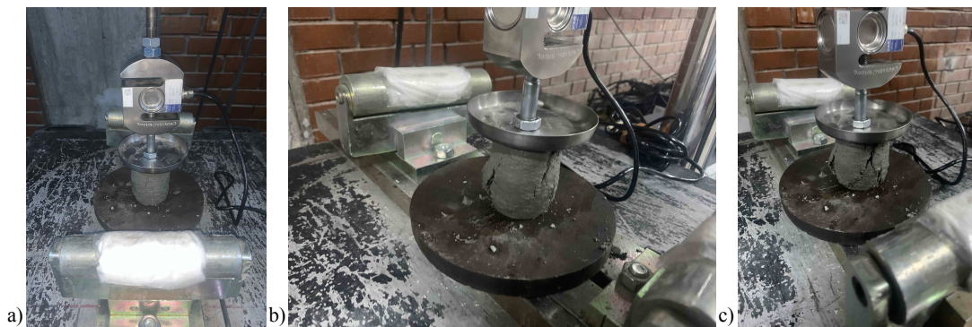
Figure 3.2: Three stages of the UUCT test, performed for a specimen at 35 minutes of age, up to a strain change of 25%.
