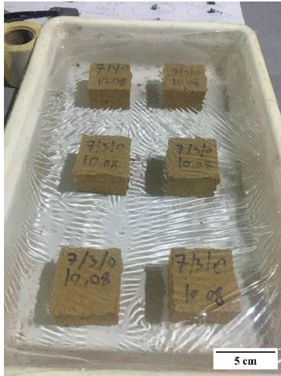
Figure 3.7 The experimental setup for water resistance testing. 5-cm COC mortar cube specimens are underwater.
