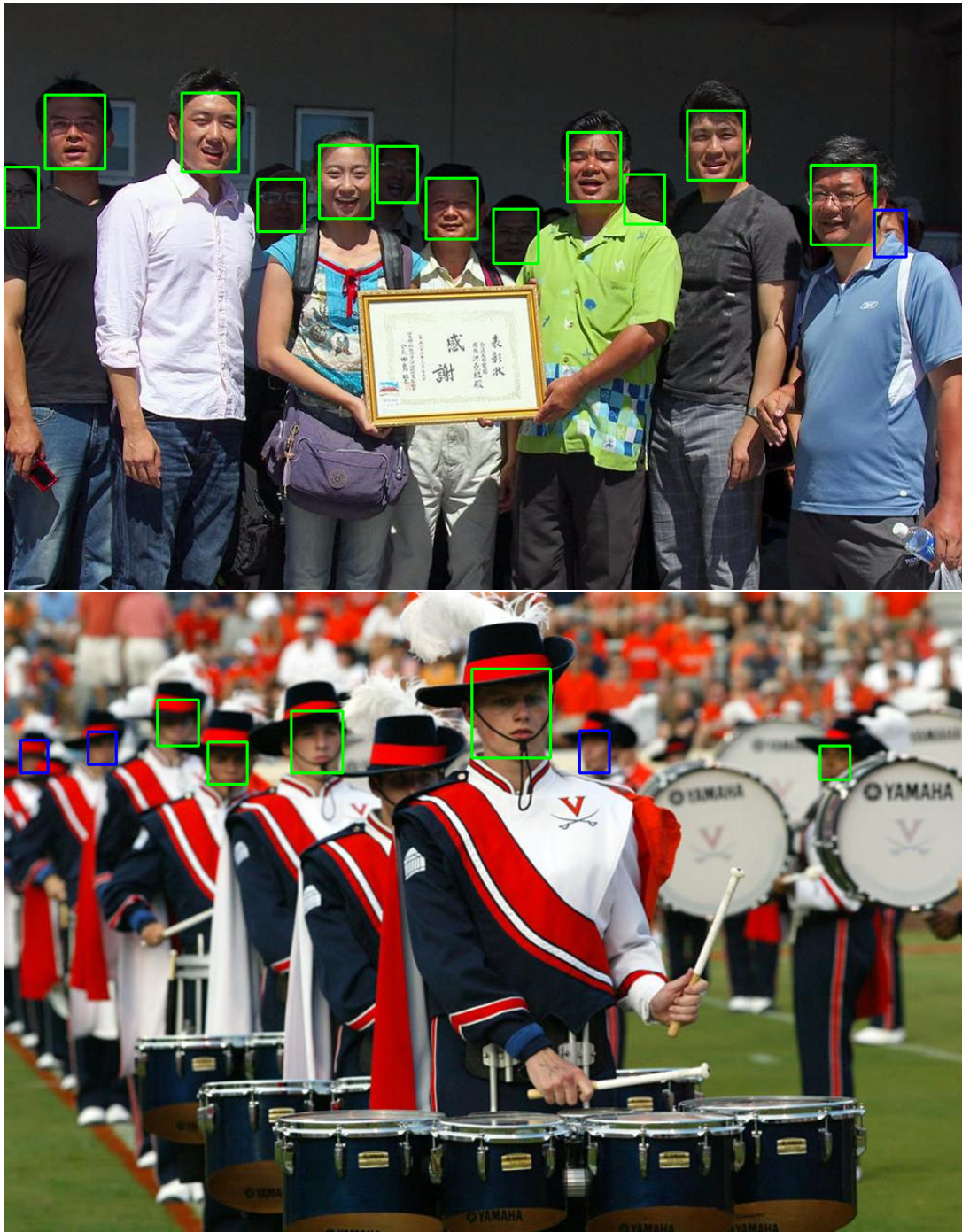
Figure 13: Qualitative results of model_finetime and model_joint were given on sample images from the Widerface [1] validation set. If the IOU of both models' predicted bounding boxes is greater than 0.5, bounding boxes are shown in green color. Blue rectangles indicate the predictions made only by the model_joint, and the bounding boxes predicted only by the model_finetime are in red.
