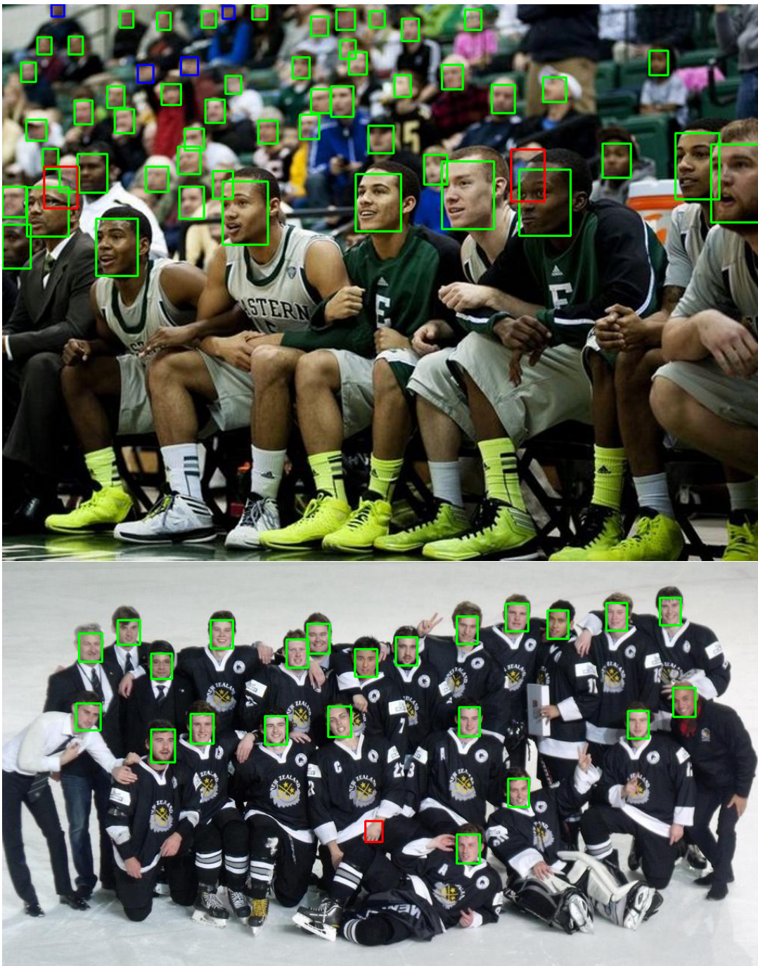
Figure 12: Qualitative results of model_freeze and model_joint were given on sample images from the Widerface [1] validation set. If the IOU of both models' predicted bounding boxes is greater than 0.5, bounding boxes are shown in green color. Blue rectangles indicate the predictions made only by the model_joint, and the bounding boxes predicted only by the model_freeze are in red.
