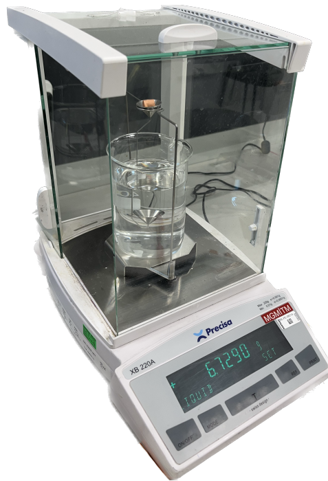
Figure 3.14: Determination of density with the Archimedes method.
