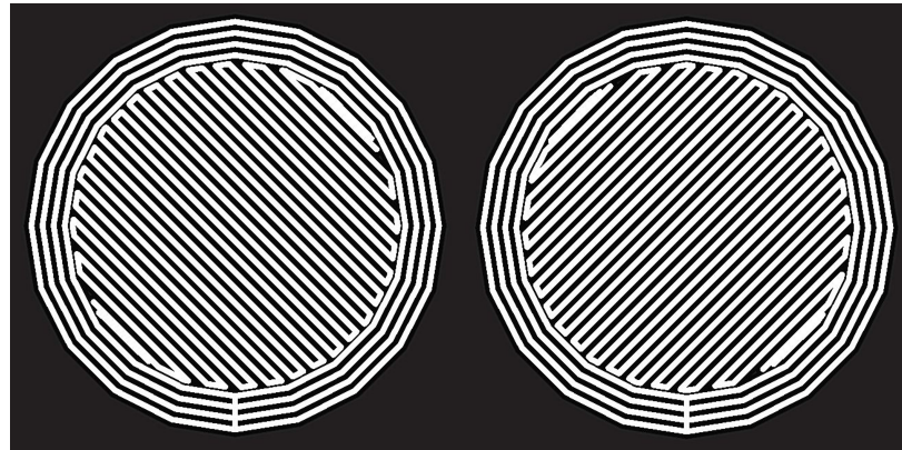
Figure 3.22: Nozzle path on the consecutive layers.
