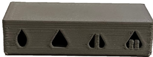
Figure 3.7: Straight test part made of 17-4 PH SS.
