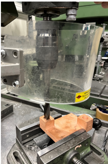
(a) Holes are enlarged with a tap drilling operation.
