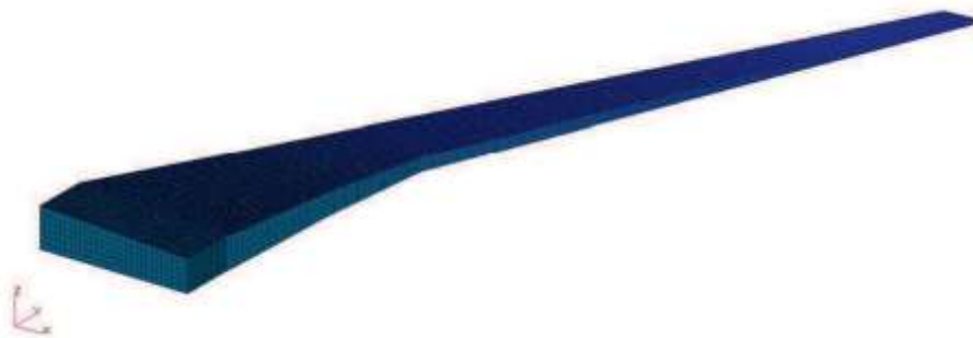
Figure 2-10 Finite Element Model of Wing Box [24]
