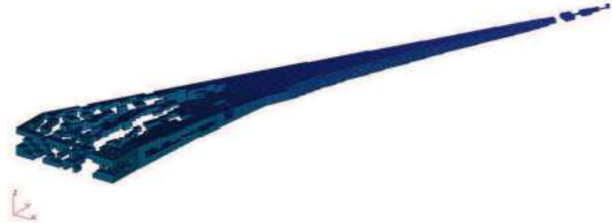
Figure 2-11 Final Topology of the Wing Box [24]
