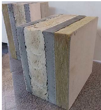
Figure 2.15. Combination of 3D concrete printed wall with traditional thermal insulation (Kaszynka et al., 2019).
