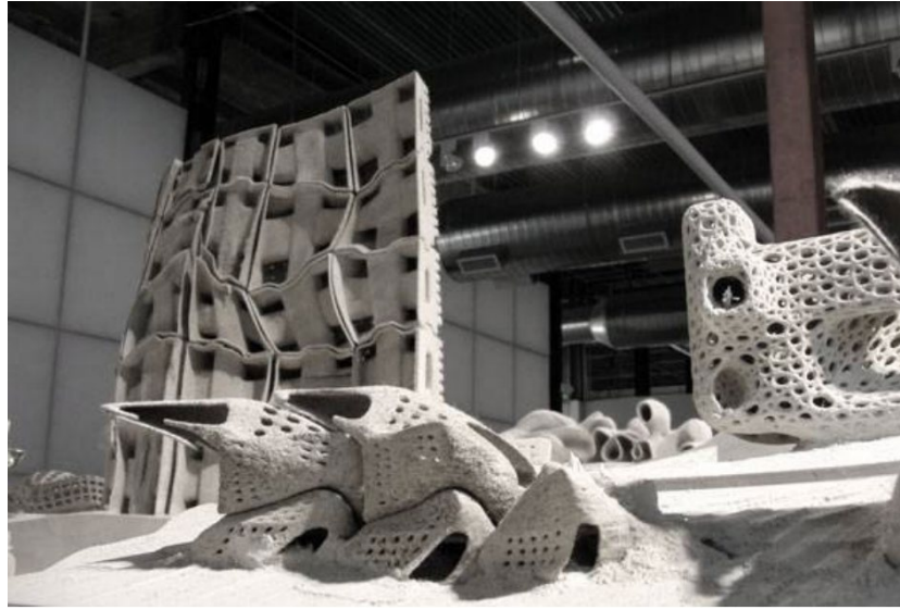
Figure 2.6. Parametric forms printed with powder bed based printing technology (Rael, 2018).
