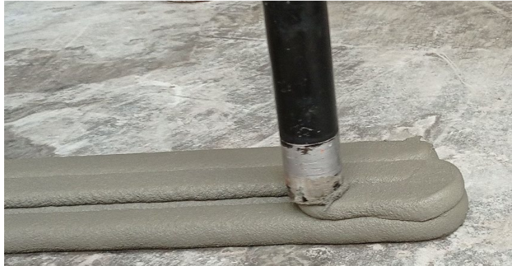
Figure 2.7. No slump 3D printable concrete printed in ISTON factory
