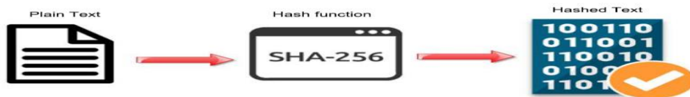
Figure 2.11. Hash function turns plain text or files to condensed hashed text (Aggarwal & Kumar, 2021)
