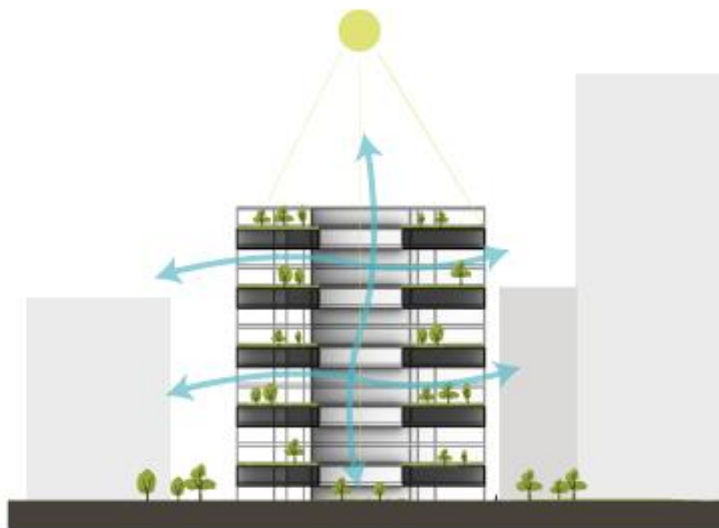
Figure 2.5. Case Study Building Section represents breezeways and transitional spaces
