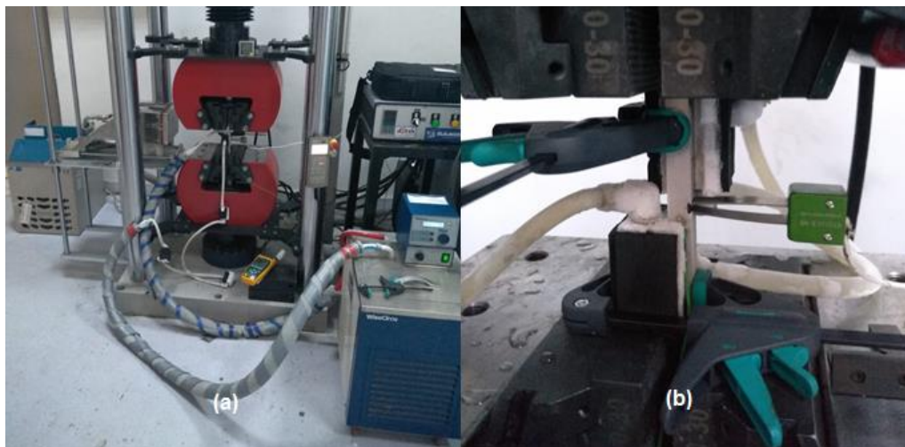
Figure 33. (a) SENT test setup and (b) specimen with attached cooling pads and clip-on-gauge.
