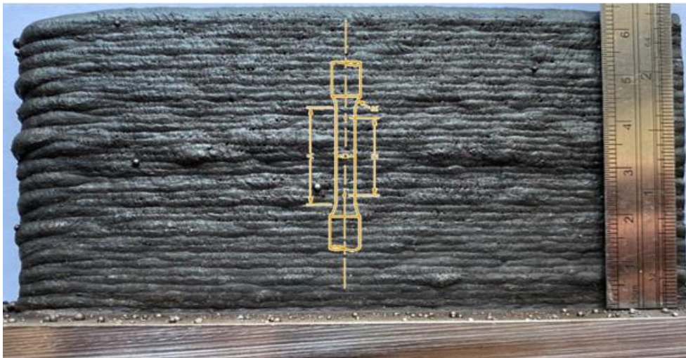
Figure 26. Extraction orientation of tensile test specimen.
