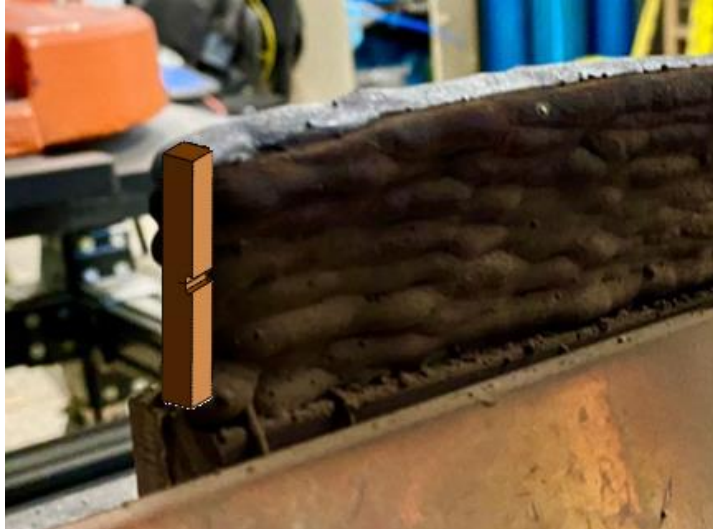
Figure 29. Orientation of fracture toughness specimens of WAAM coupons.
